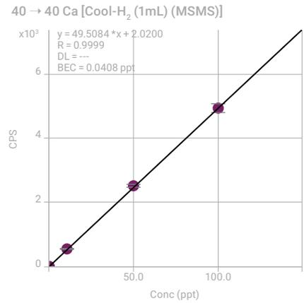
**Figure 2.** MSA calibration plot for Ca using MS/MS mode with H<sub>2</sub> flow of 1 mL/min.
