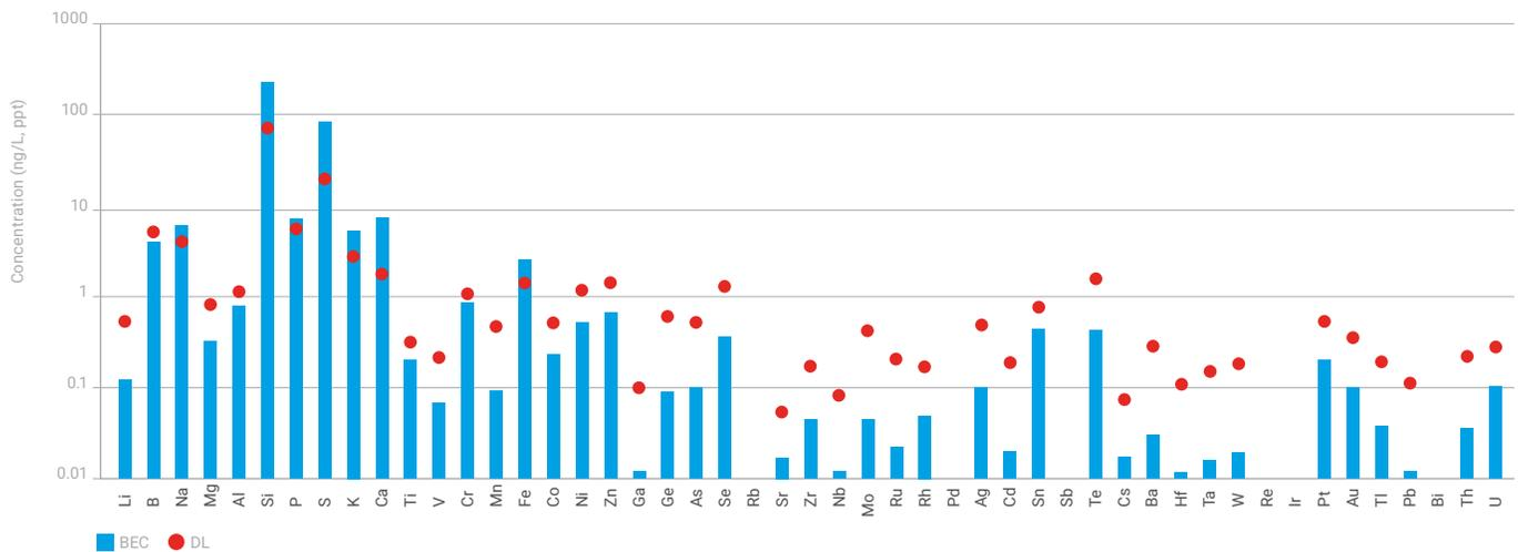
**Figure 2.** BECs and 3 $\sigma$  DLs for 49 elements in 5% HNO<sub>3</sub> blank. The BEC and DL for Rb, Pd, Sb, Re, Ir, and Bi could not be calculated, as the measured counts were zero in all replicates of the blank.
