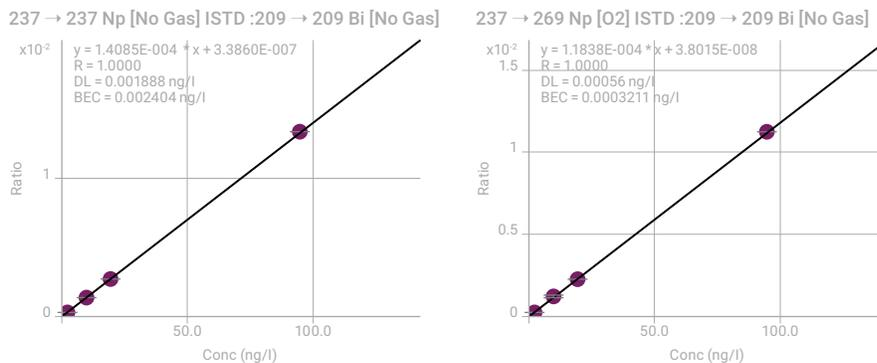
**Figure 3.** Np calibration in a 10 ppm U matrix. Left: no gas mode. Right: O<sub>2</sub> reaction gas mode – showing a 7.5x reduction in BEC. All UH-based interferences were avoided by measuring <sup>237</sup>N as <sup>237</sup>Np<sup>16</sup>O<sub>2</sub>.
