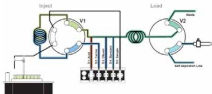
**3. Sample injection:** The prepared sample is introduced into the ICP-QQQ via the carrier solution pumped by S2. S2 provides a precise flow rate regardless of sample type. The V1 loop is washed simultaneously.
