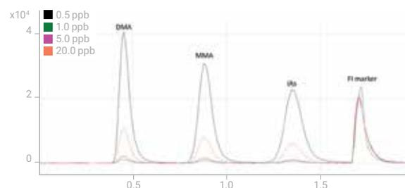
**Figure 1.** Overlay of the 0.5, 1.0, 5.0, and 20.0 µg/kg As species calibration standards. An AB internal standard (flow injection marker; fourth peak) was added post column via an external switching valve.
