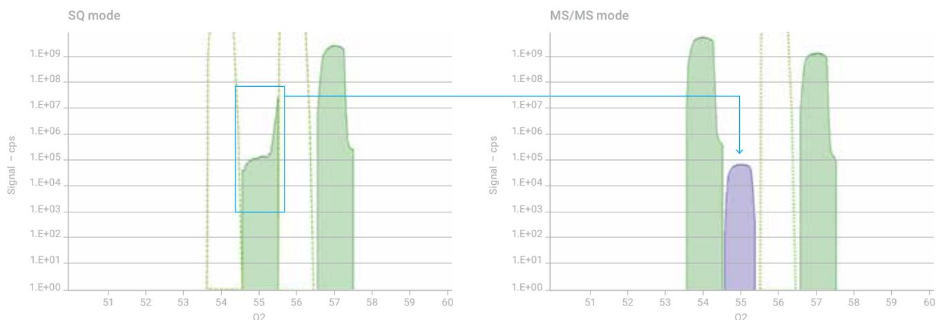
**Figure 1.** Comparison of no gas mode spectra for 500 ppm Fe solution, measured in SQ mode (left) and MS/MS mode (right). The signal colored blue was obtained in pulse counting while the green signal was obtained in analog mode. The dotted lines indicate over-range peaks (automatically skipped to protect the EM detector).
