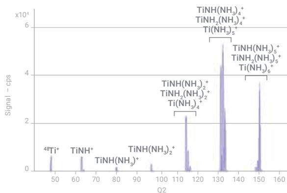
**Figure 1.** Product ion scan for <sup>48</sup>Ti<sup>+</sup> in NH<sub>3</sub> mode.
