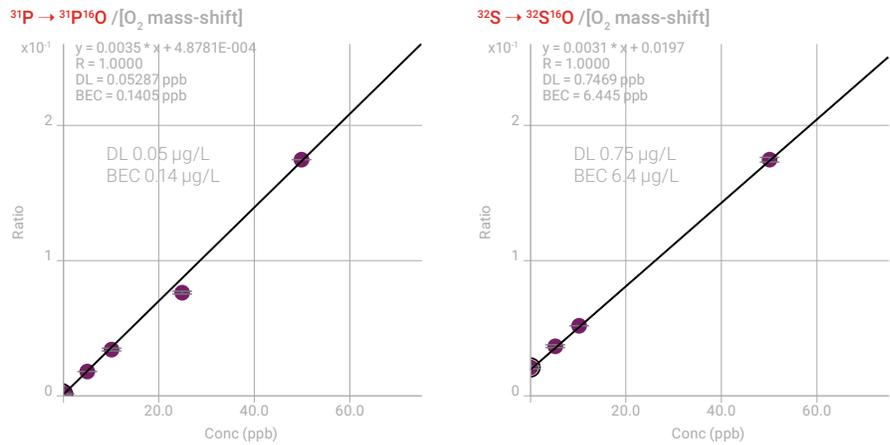
**Figure 2.** Calibration curve for P (left) and S (right) in 0.1% Fe matrix, obtained using O<sub>2</sub> mass-shift mode under robust plasma conditions.
