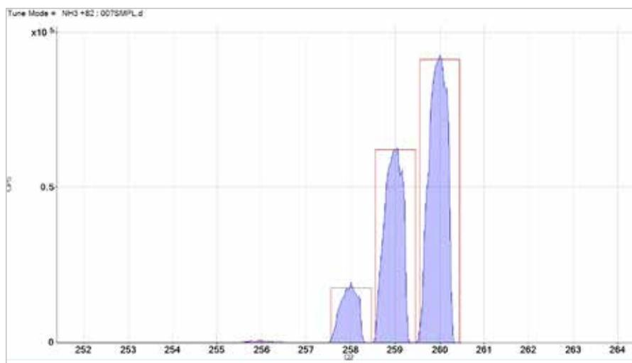
**Figure 4.** Neutral Gain Scan of the Hf isotopes as  $\text{Hf}(\text{NH})(\text{NH}_2)(\text{NH}_3)_3^+$  clusters; theoretical Hf isotopic abundances are shown in red, confirming that the isotope ratios are preserved in the product ion spectrum
