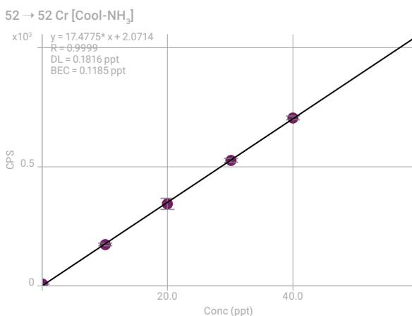
**Figure 1.** <sup>52</sup>Cr calibration curve obtained using cool plasma and NH<sub>3</sub> cell gas, showing low BEC and good linearity.
