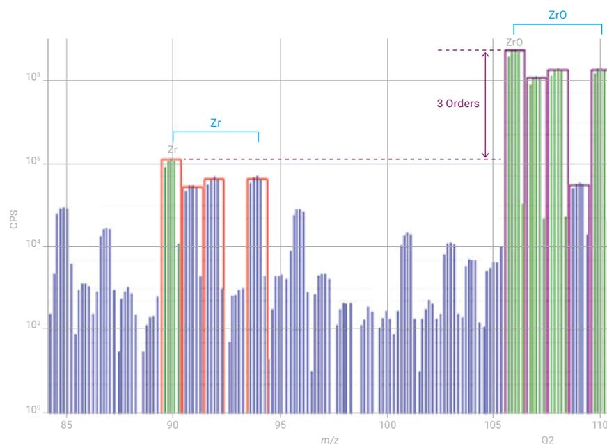
**Figure 2.** Spectrum of 10 ppm Zr obtained using Single Quad mode A with O<sub>2</sub> mass-shift-method
