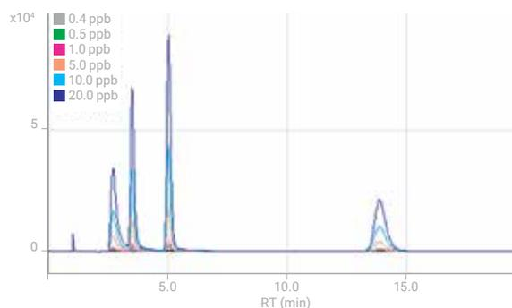
**Figure 1.** Overlaid chromatograms of As species standards at nominal concentrations of 0.4, 0.5, 1, 5, 10, 20  $\mu\text{g}/\text{kg}$  showing good peak separation. The 40  $\mu\text{g}/\text{kg}$  standard is not shown, to allow the lower concentration levels to be seen.
