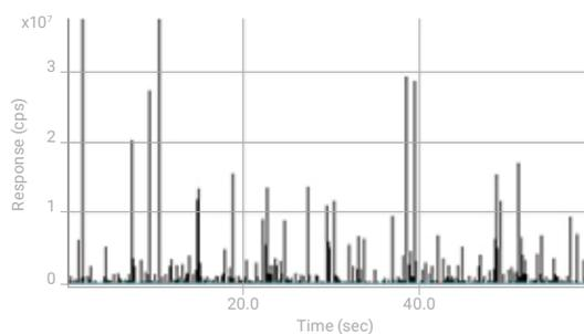
**Figure 1.** Time resolved signal for NIST 1898 TiO<sub>2</sub> NP reference material. The blue line represents a baseline automatically set by the MassHunter software function.
