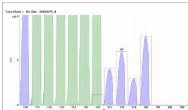
**Figure 1.** Hf (red peak template) in the presence of Lu and Yb matrix. The poor template fit for  $^{176}\text{Hf}$  (highlighted in blue outline) is due to the contribution from  $^{176}\text{Lu}$  and  $^{176}\text{Yb}$  to the signal at  $m/z$  176.
