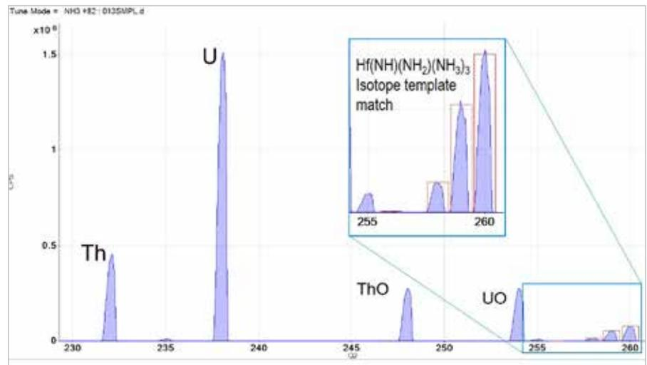
**Figure 6.** Mass spectrum of the mineral sample measured using  $\text{NH}_3$  mass-shift mode for Hf and on-mass mode for all other isotopes. The Hf isotopic pattern illustrates that all of the interferences that occurred in Single Quad mode (shown in Figure 5) have been resolved.
