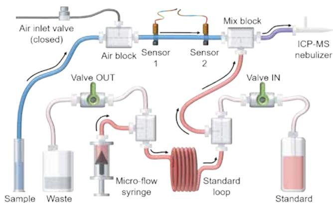
*Worked example: Addition of a 50 ppt MSA spike to a sample flowing at 200  $\mu\text{L}/\text{min}$ .*
