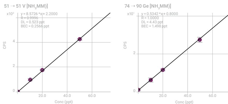
**Figure 1.** Calibration curves of V (NH<sub>3</sub> on-mass mode) and Ge (NH<sub>3</sub> mass-shift mode) in 20% HCl.
