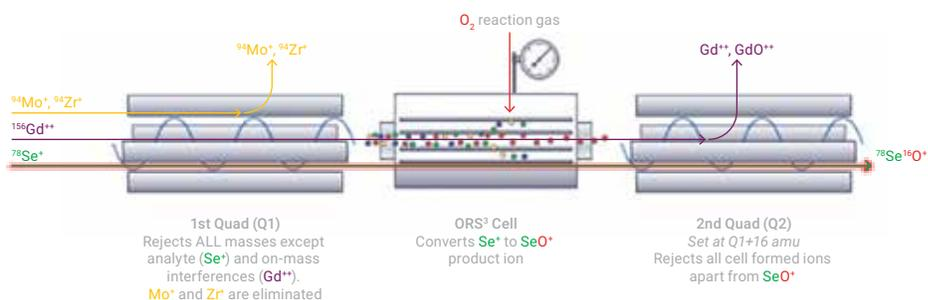
**Figure 1.** Representation of ICP-QQQ setup with Q1 set to 78 amu and Q2 set to 94 amu. Mo and Zr-based interferences are eliminated by Q1 and Gd<sup>++</sup> is eliminated by Q2 allowing the measurement of <sup>78</sup>Se as <sup>78</sup>Se<sup>16</sup>O<sup>+</sup>.
