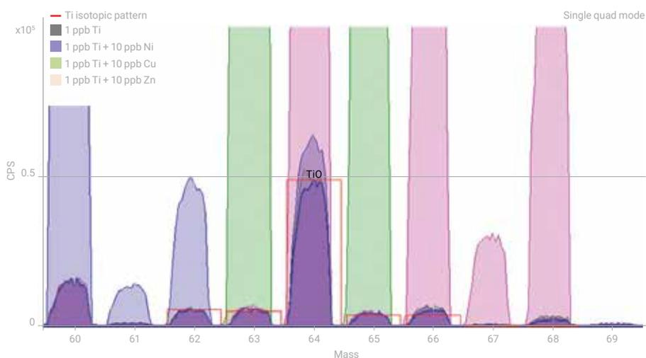
**Figure 1.** Overlaid spectra for  $TiO^+$  product ions in variable samples measured using SQ mode (see text for sample composition).
