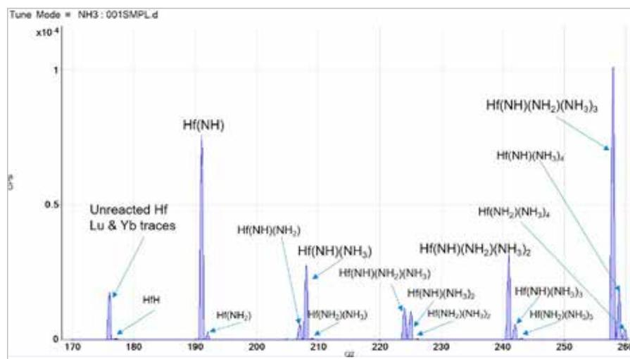
**Figure 2.** Product Ion Scan from  $m/z$  170 to  $m/z$  260 showing ammonia adduct reaction product ions formed from  $^{176}\text{Hf}$  precursor ion (Q1 set to  $m/z$  176)
