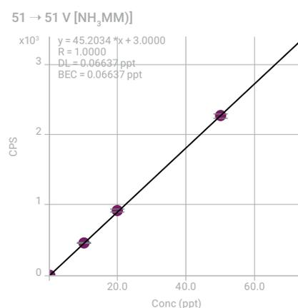
Figure 2. Calibration curve of V in 9.8%  $\text{H}_2\text{SO}_4$ .
