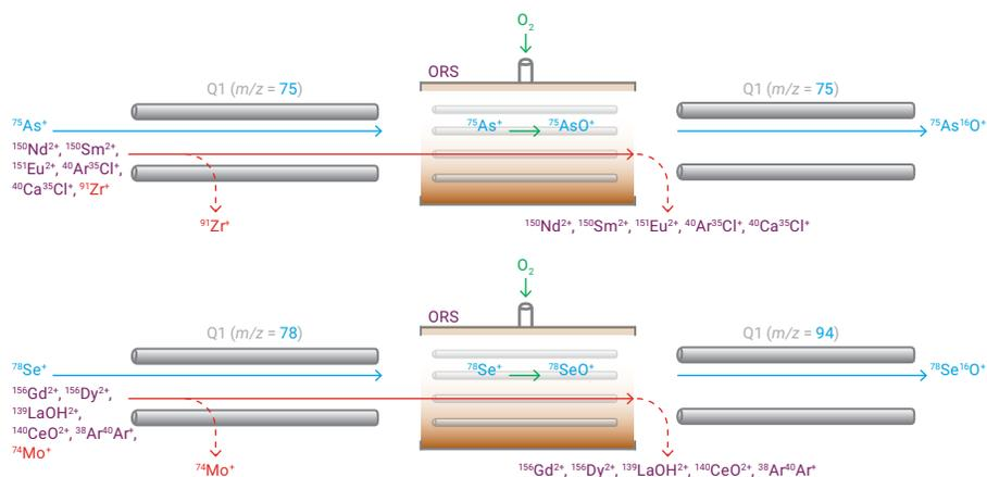
Figure 1. ICP-QQQ MS/MS  $O_2$  mass-shift method for measuring  $^{75}\text{As}$  (top) and  $^{78}\text{Se}$  (bottom)
