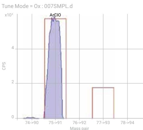
**Figure 5.** Neutral gain scan spectrum for 20% high purity HCl showing the theoretical isotope template for  $^{40}\text{Ar}^{35}\text{Cl}^{16}\text{O}^+$  and  $^{40}\text{Ar}^{37}\text{Cl}^{16}\text{O}^+$ . Q1 was scanned from  $m/z$  74 to 78, while Q2 was set to Q1 + 16.
