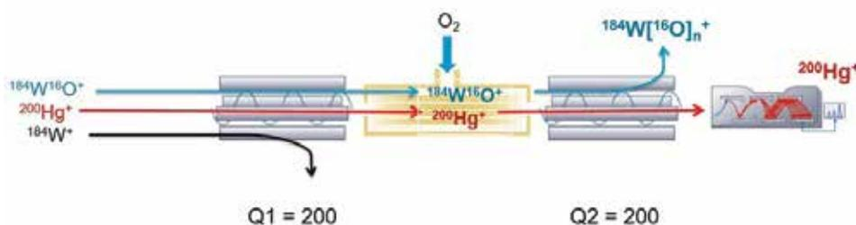
**Figure 2.** Reaction mechanism in MS/MS mode with O<sub>2</sub> cell gas for removal of WO<sup>+</sup> overlap to allow on-mass detection of Hg in a tungsten matrix. The same mechanism is also effective at resolving WOH<sup>+</sup> overlaps.
