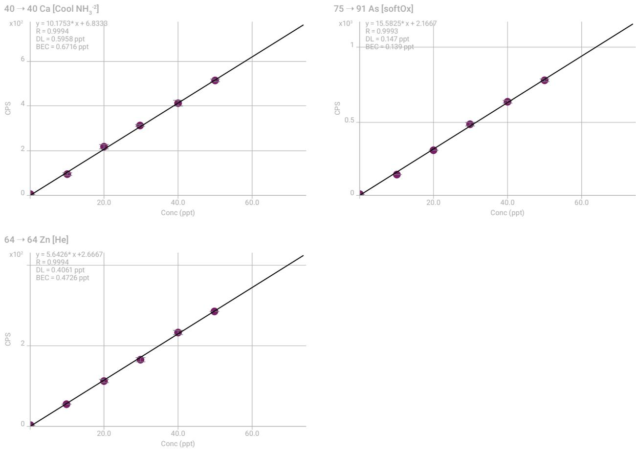
Figure 3. Calibration plots for Ca, Zn, and As in H<sub>2</sub>O<sub>2</sub>. All values in ng/L (ppt).
