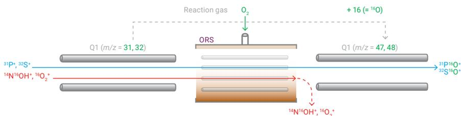
**Figure 1.** Mechanism of MS/MS mass-shift mode ( $Q2 = Q1+16$ ) using  $\text{O}_2$  reaction gas for the measurement of P as  $^{31}\text{P}^{16}\text{O}^+$  and S as  $^{32}\text{S}^{16}\text{O}^+$  at  $m/z$  47 and 48 respectively.
