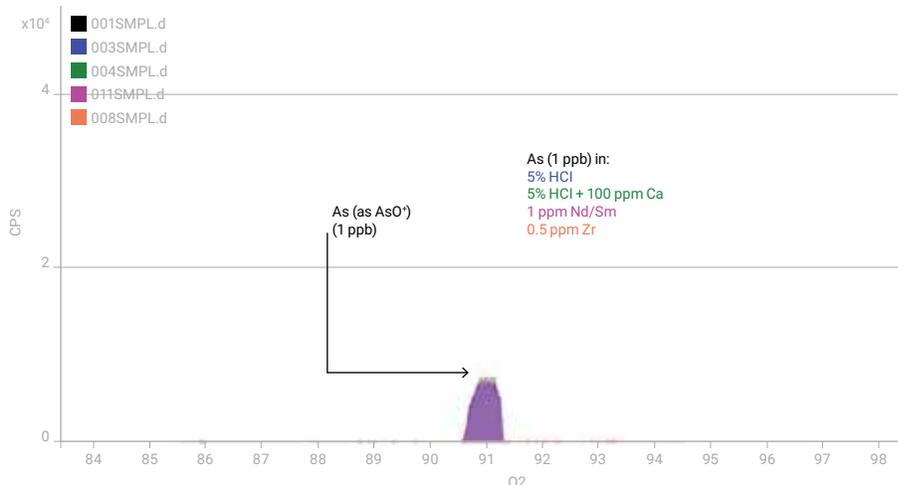
**Figure 3.** MS/MS mass-shift with O<sub>2</sub> reaction mode provides consistent, interference-free measurement of As as AsO in all the matrices.
