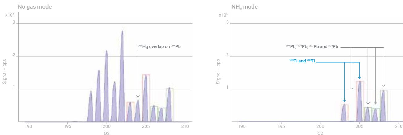
**Figure 1.** Standard solution (1 ppb each of Pb and Tl) spiked with 10 ppb Hg without cell gas (left) and with NH<sub>3</sub> (right) using MS/MS mode. Note the <sup>204</sup>Hg interference on <sup>204</sup>Pb in no gas mode.
