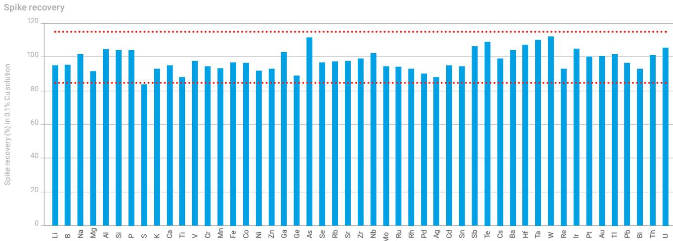
**Figure 4.** Spike recovery test at 50 ppt (200 ppt for S, P, and Si) in 0.1% Cu solution. Most elements were within 90–110% recovery. The red lines indicate upper and lower limits of 85 to 115% recovery.
