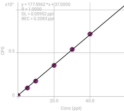
Figure 1. Calibration curves for several SEMI specification elements in high purity 68% HNO<sub>3</sub>.
