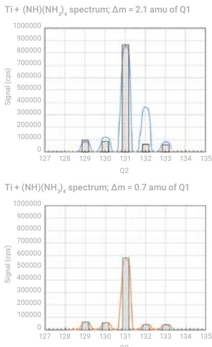
**Figure 2.** Ti + (NH)(NH<sub>3</sub>)<sub>4</sub> product ion spectrum of five Ti isotopes obtained with NH<sub>3</sub> cell gas mode: <sup>46</sup>Ti (8.25%), <sup>47</sup>Ti (7.44%), <sup>48</sup>Ti (73.72%), <sup>49</sup>Ti (5.41%), and <sup>50</sup>Ti (4.29%). A Ti standard solution was analyzed using ICP-QQQ with NH<sub>3</sub> cell gas. Top: Q1 was set at Δm = 2.1 amu. Bottom: spectrum was acquired with Q1 set at Δm = 0.7 amu.
