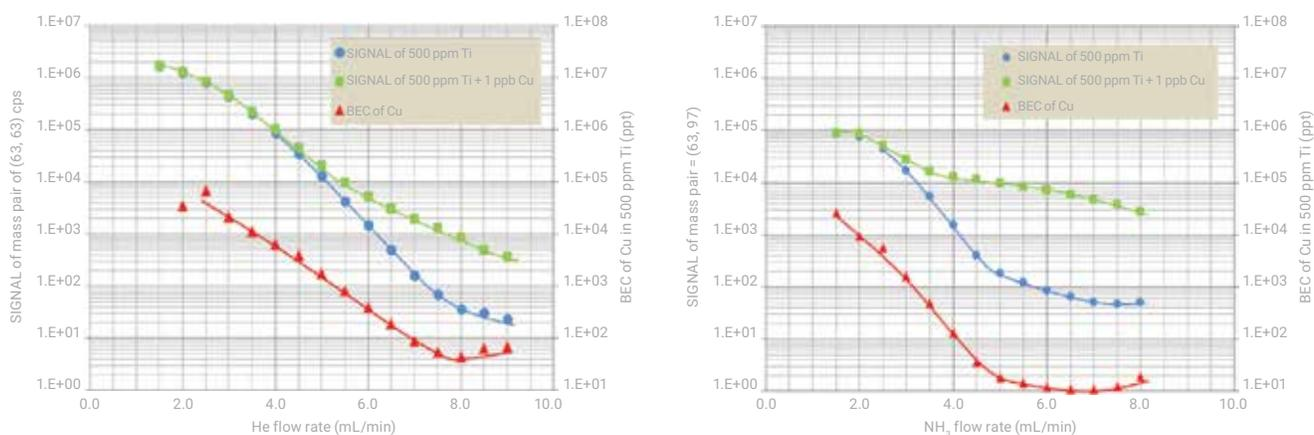
**Figure 1.** (Left) Cu signal (mass pair 63, 63) vs. He cell gas flow rate, for 500 ppm Ti matrix unspiked and with 1 ppb Cu spike, and calculated BEC. (Right) Cu signal (mass pair 63, 97) vs.  $\text{NH}_3$  cell gas flow rate, for 500 ppm Ti matrix unspiked and with 1 ppb Cu spike, and calculated BEC.
