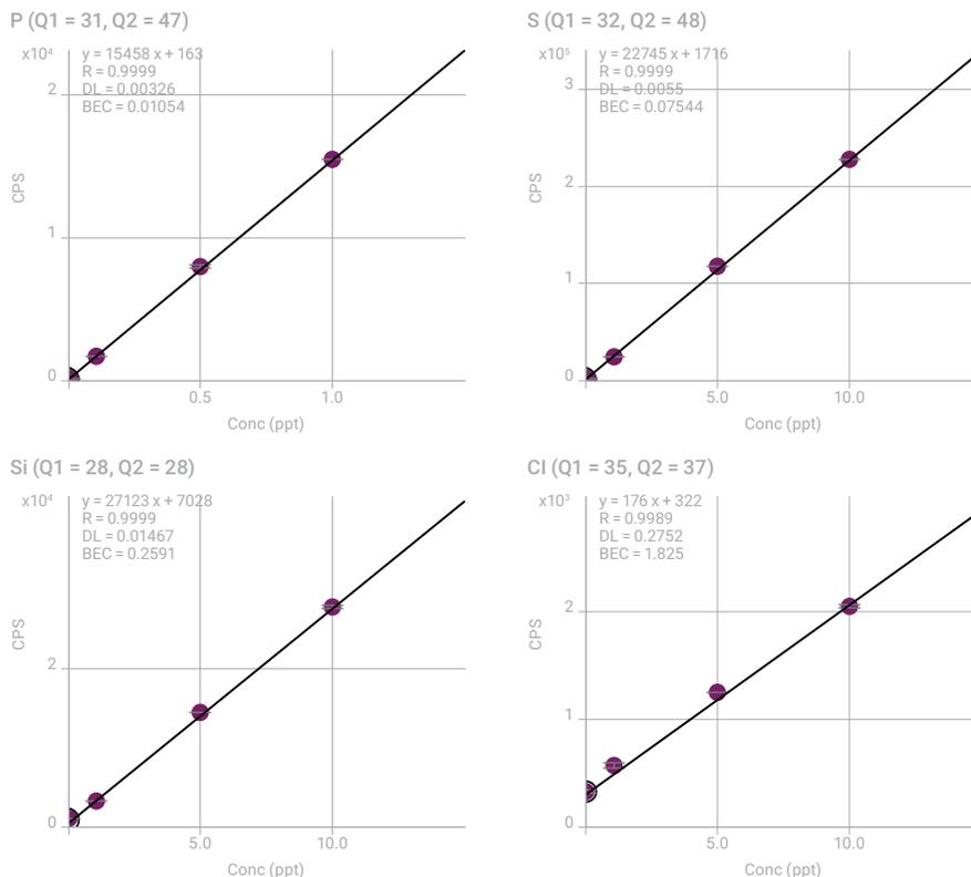
**Figure 1.** Calibration plots of P, S, Si, and Cl in UPW. All values in ug/L (ppb).
