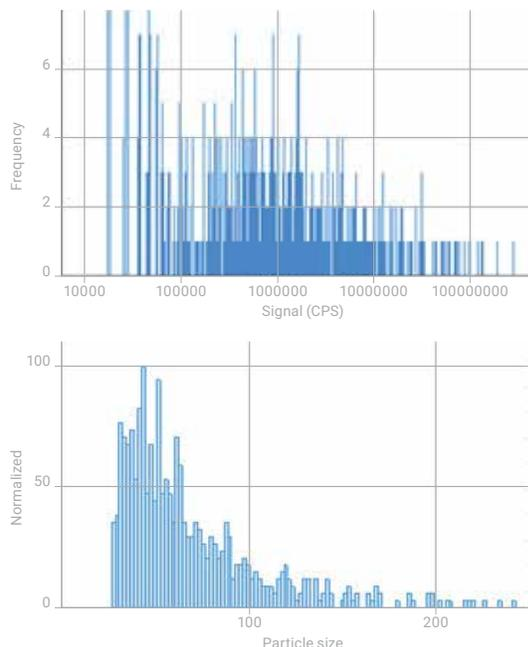
**Figure 2.** Signal frequency distribution (upper) and particle size distribution (lower) for NIST 1898 TiO<sub>2</sub> NP reference material.
