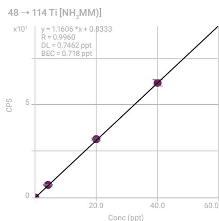
Figure 1. Calibration curve of Ti in 9.8%  $\text{H}_2\text{SO}_4$ .
