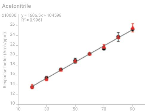
**Figure 1.** Measured response curve demonstrating the effect of the organic solvent (acetonitrile) content of the mobile phase on the Cl response of ICP-QQQ for both inorganic Cl and diclofenac-Cl (95% confidence intervals, n = 3). The response factor was found to be independent of the chemical form, as expected.
