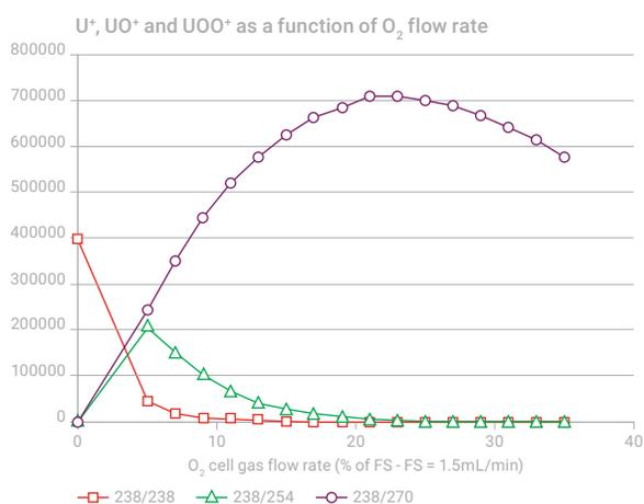
**Figure 1.** U<sup>+</sup> (238 → 238), UO<sup>+</sup> (238 → 254), and UO<sub>2</sub><sup>+</sup> (238 → 270) as a function of O<sub>2</sub> cell gas flow rate.
