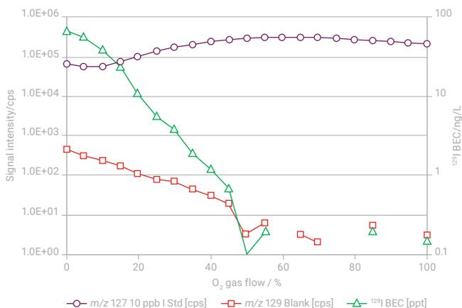
**Figure 1.** Profile of <sup>127</sup>I<sup>+</sup>, <sup>129</sup>Xe<sup>+</sup> signals and estimated <sup>129</sup>I BEC. For the BEC calculation, the sensitivity of <sup>129</sup>I was assumed to be the same as <sup>127</sup>I. Scale of O<sub>2</sub> flow: 100% = 1.12 mL/min.
