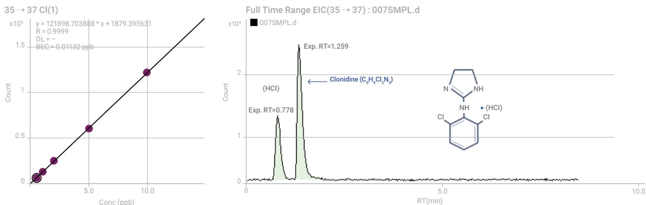
**Figure 3.** (Top) Calibration curve for Cl (measured as <sup>35</sup>ClH<sub>2</sub><sup>+</sup>) in clonidine hydrochloride (C<sub>9</sub>H<sub>9</sub>Cl<sub>2</sub>N<sub>3</sub>·HCl) standards. (Bottom) Chromatogram of clonidine hydrochloride in Catapres® sample.
