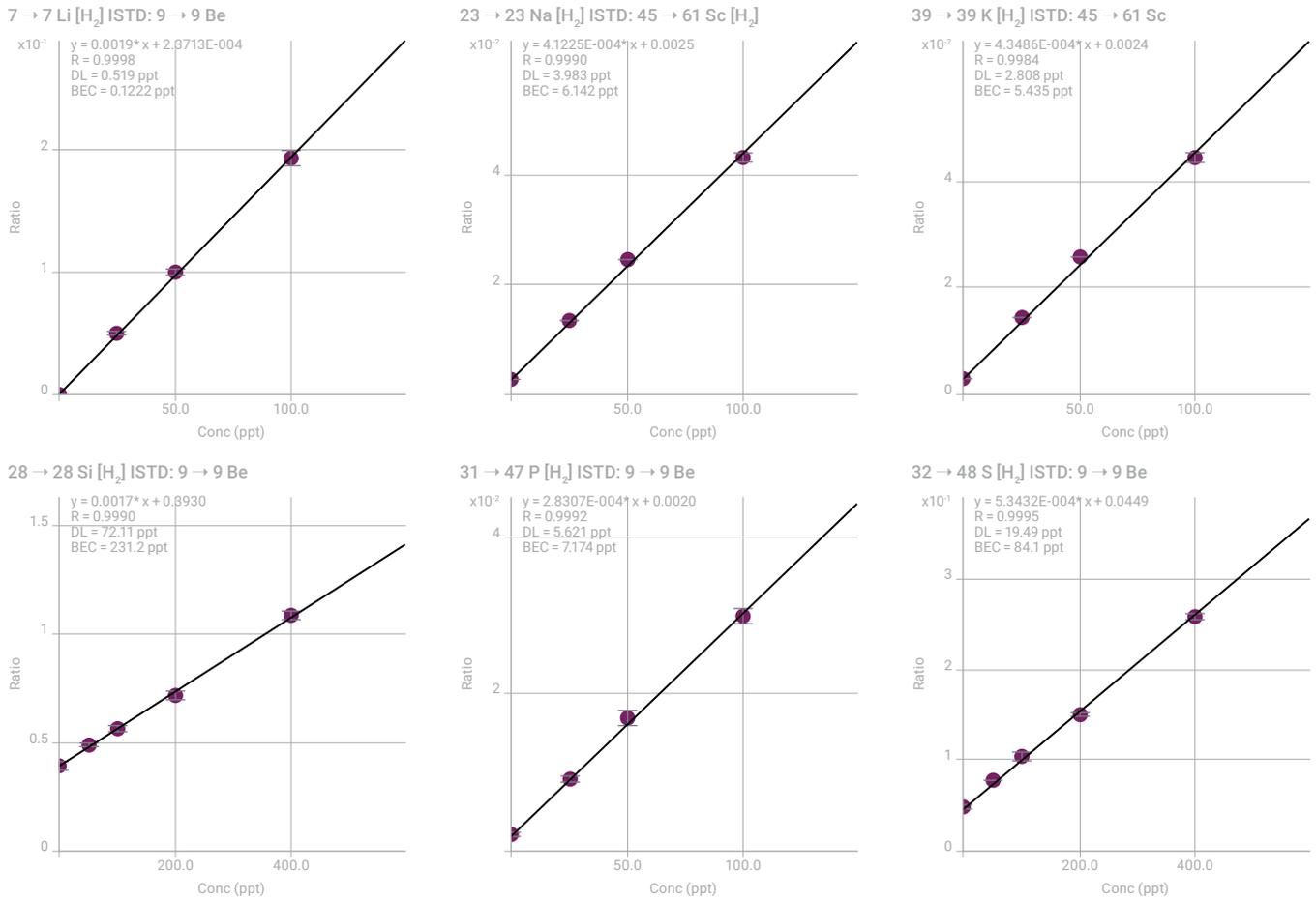
Figure 1. Calibrations for easily-ionized elements Li, Na, and K, and challenging elements Si, P, and S.
