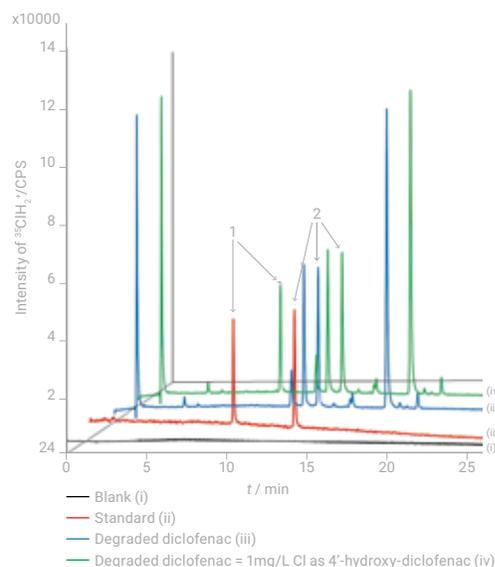
**Figure 2.** Chlorine chromatograms for (i) a blank, (ii) 4'-hydroxydiclofenac plus diclofenac, each at a concentration equivalent to 1 mg/L Cl, (iii) synthetically degraded diclofenac at 10 mg/L Cl, and (iv) synthetically degraded diclofenac at 10 mg/L Cl, spiked with 4'-hydroxydiclofenac at 1 mg/L Cl. Peak 1: 4'-hydroxydiclofenac; peak 2: diclofenac; other peaks: degradation products with unknown chemical structure.
