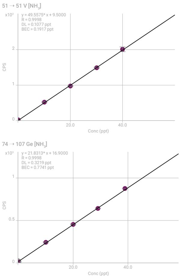
Figure 3. <sup>51</sup>V and <sup>74</sup>Ge calibration curve obtained using NH<sub>3</sub> cell gas.
