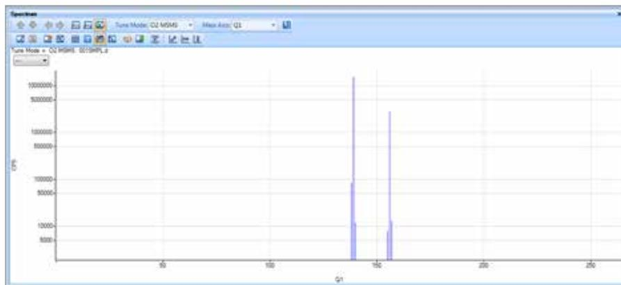
**Figure 3.** Precursor ion scan from 2-260 amu for product ion mass 156, in a 50 ppm La matrix. Six peaks are seen at *m/z* = 138, 139, 140, 155, 156 and 157, with the intense peaks at *m/z* 139 and *m/z* 156 being due to <sup>139</sup>La<sup>+</sup> and <sup>139</sup>La<sup>16</sup>O<sup>+</sup>H<sup>+</sup> respectively.
