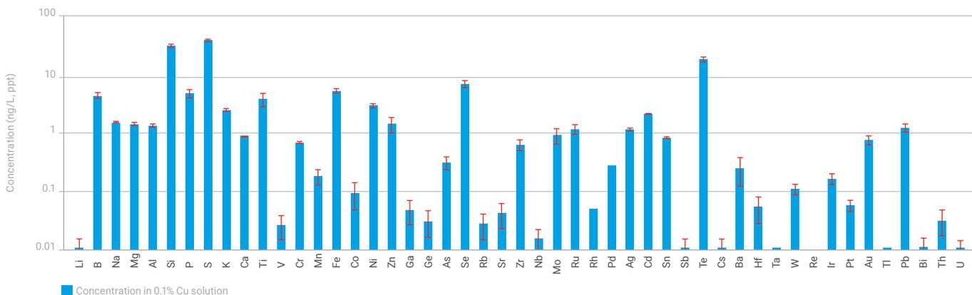
**Figure 3.** Measured concentrations of 49 elements in 0.1% 9N Cu sample (error bars = standard deviation for three samples). The values shown in ng/L (ppt) in solution) are equivalent to the values in  $\mu\text{g}/\text{kg}$  (ppb) in the original solid metal. The concentration reported for Re was 0.000 ppt. SDs were zero for Rh, Pd, Ta, Re, and Tl.
