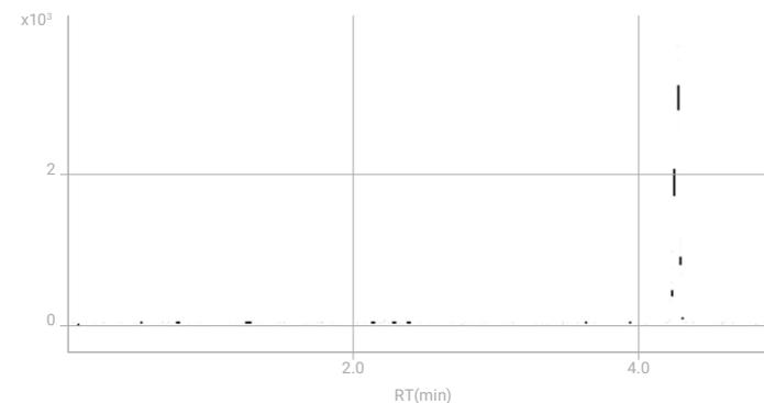
**Figure 2.** Chromatogram of 0.4 ppb  $\text{PH}_3$  standard. S/N: 96.9.
