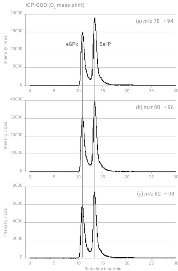
**Figure 1.** Elution profiles of Se in rat serum. A 200- $\mu$ L aliquot of a rat serum sample was injected into a GS-520HQ column and the eluate was monitored by ICP-QQQ (a-c) at  $m/z$  94 (a), 96 (b), and 98 (c).
