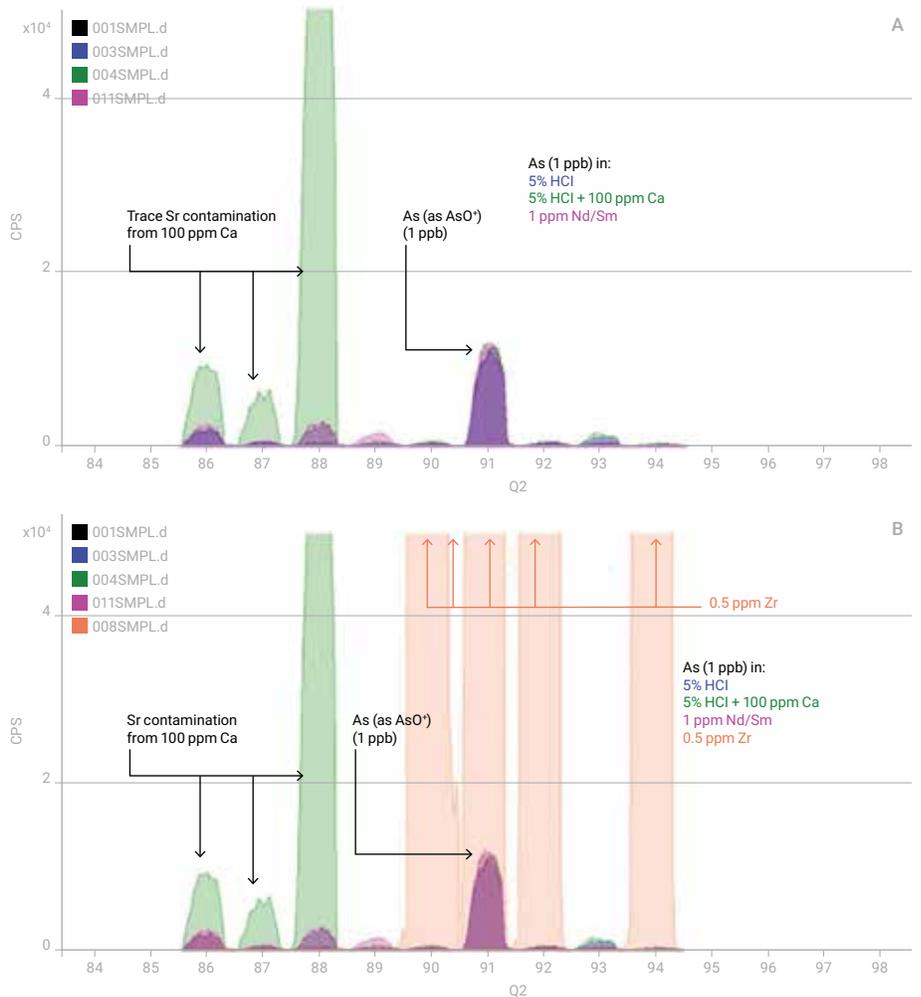
**Figure 2. a)** Nd<sup>++</sup> and Sm<sup>++</sup> interferences at *m/z* 75 are avoided in SQ O<sub>2</sub> reaction mode, by measuring As as the AsO<sup>+</sup> product ion at *m/z* 91; **b)** SQ O<sub>2</sub> reaction mode fails to remove <sup>91</sup>Zr<sup>+</sup> overlap on the AsO<sup>+</sup> product ion.
