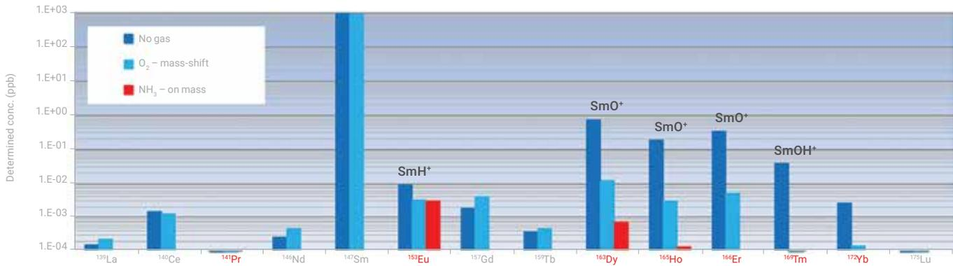
**Figure 2.** Measured concentration of REE impurities in 1 ppm Sm solution. Sm based interferences are observed on Eu, Dy, Ho, Er, Tm and Yb. Only the elements in red were measured in NH<sub>3</sub> on-mass mode.
