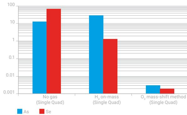
**Figure 2.** BEC of As and Se in 1ppm REE mixed solution with three measurement modes: no gas, H<sub>2</sub> on-mass and O<sub>2</sub> mass-shift mode.
