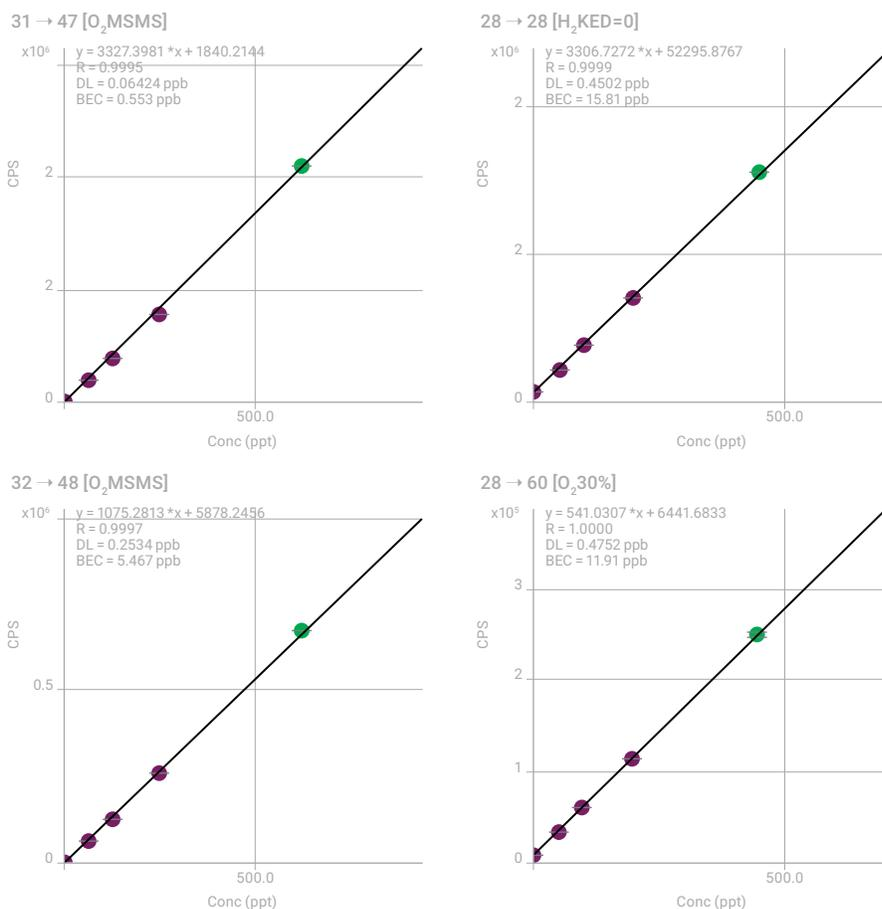
Figure 1. Calibration curve using MS/MS with O<sub>2</sub> mass-shift for P (top) and S (bottom) in NMP.
