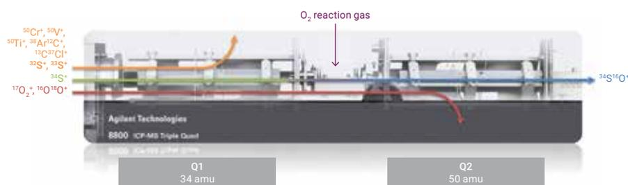
**Figure 1.** Mechanism of MS/MS mass-shift for sulfur isotope analysis. The mass difference between Q1 and Q2 is fixed at 16 amu, so only the + <sup>16</sup>O-atom transition is observed – the other oxygen isotope transitions are eliminated so the original sulfur isotopic pattern is preserved.
