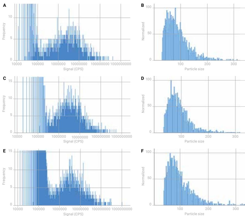
**Figure 3.** TiO<sub>2</sub> NP measurement of commercial sunscreen using ICP-QQQ. Signal distribution A) and particle distribution B) of sunscreen dispersed in de-ionized water. Signal distribution C) and particle distribution D) of sunscreen dispersed in tap water. Signal distribution E) and particle distribution F) of sunscreen dispersed in the matrix mixture.
