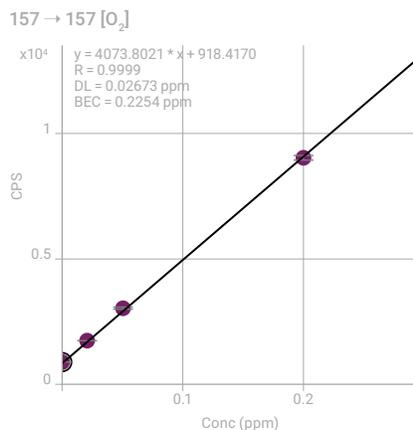
**Figure 1.** Calibration curve for F measured as BaF<sup>+</sup> in O<sub>2</sub> mode.
