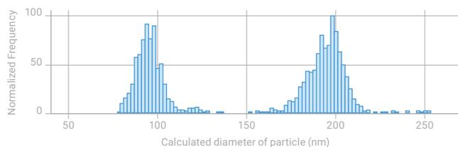
**Figure 2.** Size distribution result of 100 and 200 nm SiO<sub>2</sub> NPs in 1% ethanol.
