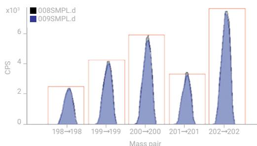
**Figure 3.** Hg isotopes with W matrix (blue shading) and without W matrix (gray shading), confirming accurate Hg isotope abundances and effective removal of W-based interferences on all Hg isotopes by ICP-QQQ with MS/MS.
