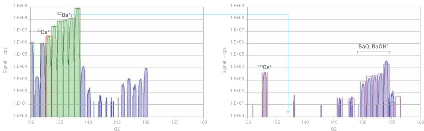
**Figure 3.** Mass spectra of a solution containing 20 ppb Cs + 5 ppm Ba: (left) SQ no gas and (right) MS/MS N<sub>2</sub>O reaction mode.
