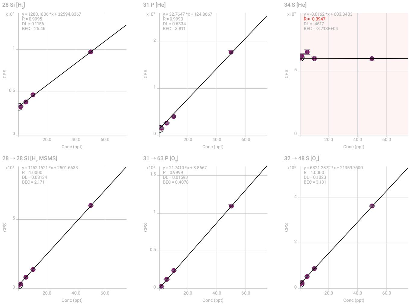
**Figure 1.** Calibration curves for Si, P and S showing SQ results (upper) compared with MS/MS results (lower). <sup>32</sup>S was not measurable at the spiked concentrations in methanol in SQ mode due to the intense <sup>16</sup>O<sub>2</sub><sup>+</sup> polyatomic interference.
