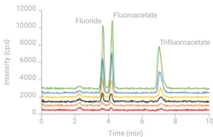
**Figure 1.** HPLC-ICP-QQQ chromatogram of fluoride, fluoroacetate, and trifluoroacetate at different F concentrations: 0.1, 0.25, 0.5, 1.0, 2.5, and 5.0 mg/L (as indicated by red to green colored lines).
