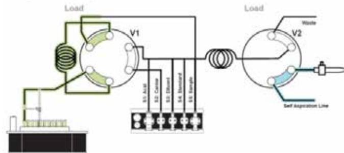
**2. Sample dilution and sample spiking:** Syringes S1, S2, S3, and S4 mix the acid, sample, diluent, and spike solution into a loop connecting V1 and V2.
