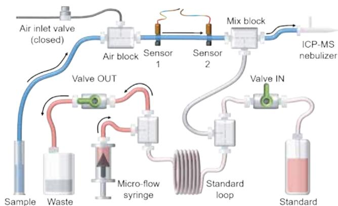
**Step 3: Sample flow rate is measured to allow calculation of MSA spike volumes.**
