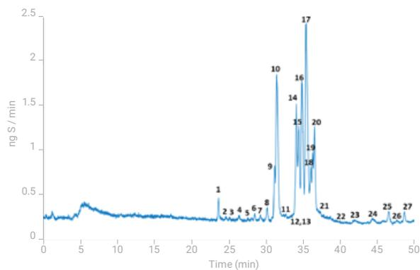
**Figure 1.** capLC-ICP-QQQ mass flow chromatogram of *Naja mossambica* venom. All the venom protein species eluted between 20 and 50 min (S detection). The 27 sulfur-containing peaks are numbered—see Table 2 for more information.
