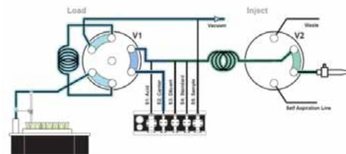
**4. Valve wash:** UPW or acidified UPW is used to clean the lines between V1 and V2.
