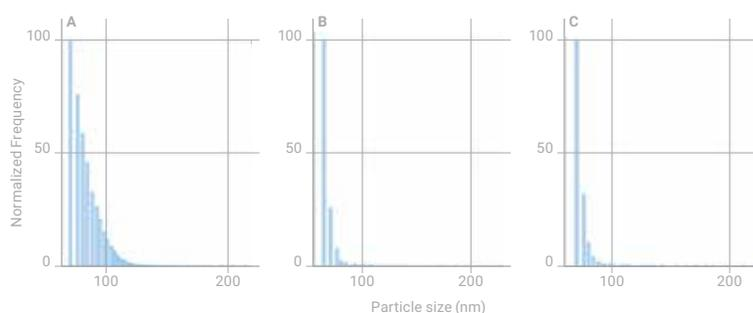
**Figure 4.** Comparison of size distributions for Mo NPs as  $\text{MoS}_2$  in the three asphaltene samples: A, B, and C. Modified with permission from J. Nelson et al., *Energy Fuels*, 2017, 31 (11), 11971–11976. © 2017 American Chemical Society.
