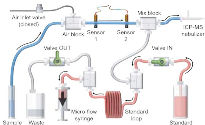
**Step 2: Excess standard solution is pumped to waste.**
