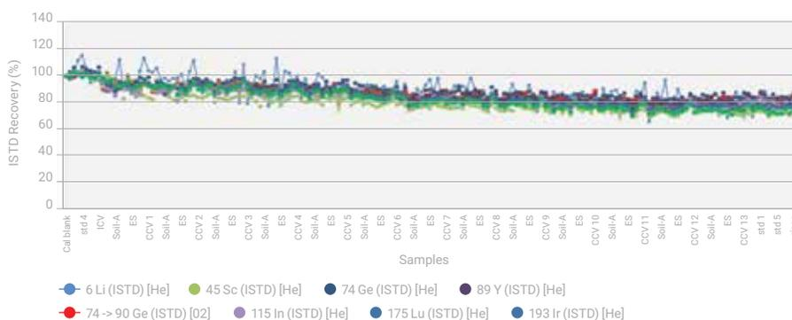
**Figure 1.** ISTD signal stability plot over 12 hours.
