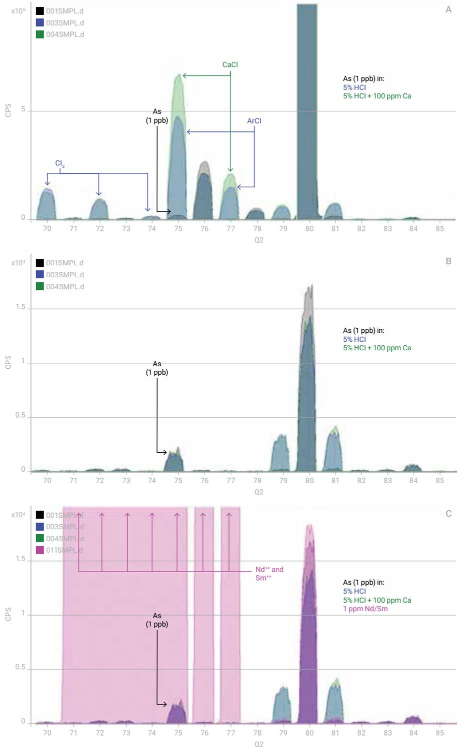
**Figure 1. a)** As<sup>+</sup> (*m/z* 75) in no gas mode, showing polyatomic interferences from ArCl<sup>+</sup> and CaCl<sup>+</sup>; **b)** ArCl<sup>+</sup> and CaCl<sup>+</sup> polyatomics are removed in He collision mode; **c)** He collision mode fails to remove Nd<sup>++</sup> and Sm<sup>++</sup> interferences at *m/z* 75.
