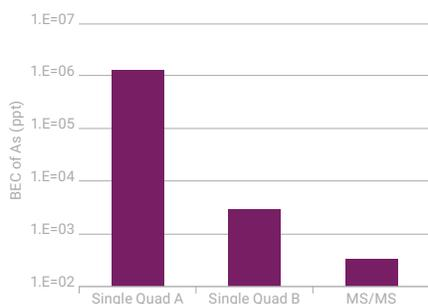
**Figure 1.** BEC of As in 1000 ppm Co solution with O<sub>2</sub> mass-shift method using three acquisition modes (note log intensity scale).
