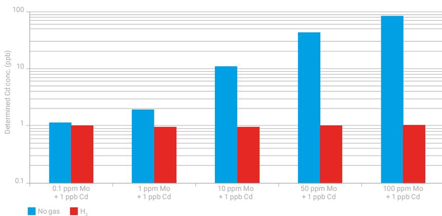
**Figure 2.** 1 ppb Cd spike recovery in a series of Mo matrix solutions using no gas mode and MS/MS H<sub>2</sub> mode.
