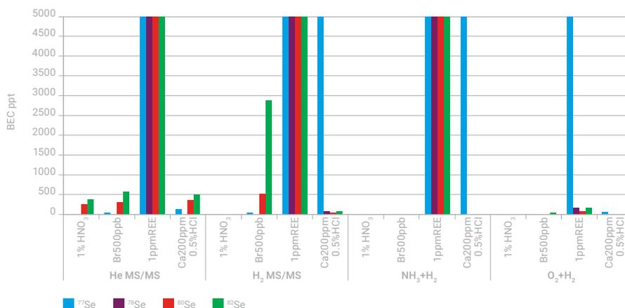
**Figure 1.** Preliminary study of the effectiveness of different cell gases for interference removal. Four synthetic matrices likely to give rise to interferences on the Se isotopes were measured using each of the 4 different cell gas modes.
