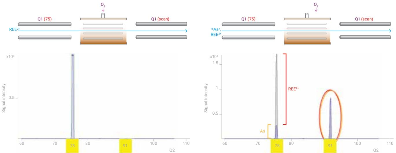
**Figure 3.** Product ion scan spectrum of O<sub>2</sub> mass-shift method. (Left) 1 ppm mixed-REE solution and (right) 1 ppm mixed-REE plus 1 ppb As spike.
