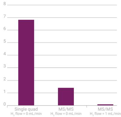
**Figure 1.** BECs for Ca obtained using Single Quad mode with no cell gas [6.8 ppt], MS/MS mode with no cell gas [1.4 ppt], and MS/MS mode with an H<sub>2</sub> cell gas flow of 1 mL/min [0.041 ppt].
