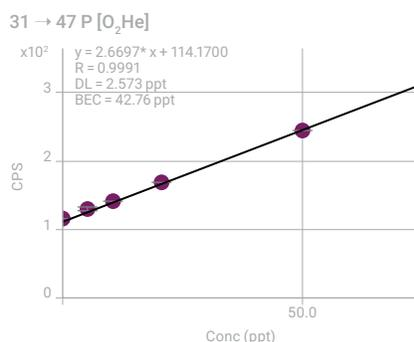
**Figure 3.** MSA calibration curve for <sup>31</sup>P.
