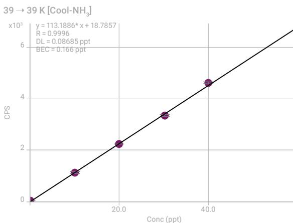
**Figure 2.** <sup>39</sup>K calibration curve obtained using cool plasma and NH<sub>3</sub> cell gas.
