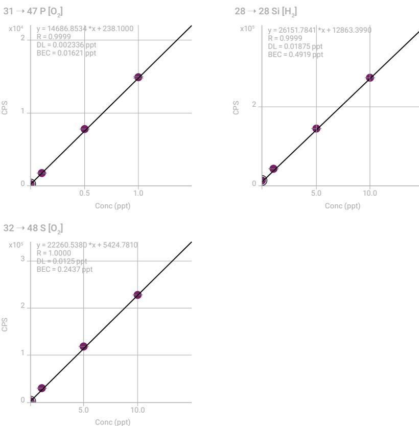
Figure 2. Calibration plots of P, S and Si in H<sub>2</sub>O<sub>2</sub>.
