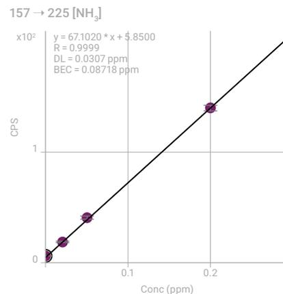
**Figure 2.** Calibration curve for F measured as BaF(NH<sub>3</sub>)<sub>4</sub><sup>+</sup> in NH<sub>3</sub> mode.
