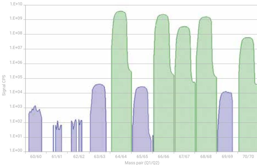
Figure 3. 1000 mg/L Zn spiked with 1  $\mu\text{g}/\text{L}$  Cu. (1 ppb: 63/total = 0.667, 65/total = 0.333, no mass bias correction performed. If there was some contribution from Zn it would influence  $m/z$  63 differently from  $m/z$  65, because of the different abundance of the Zn isotopes).
