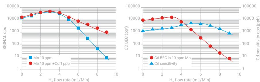
**Figure 1.** (Left): Signal for  $m/z$  111 with 10 ppm Mo and 10 ppm Mo + 1 ppb Cd, plotted as a function of H<sub>2</sub> flow rate. (Right): Estimated Cd BEC in the presence of 10 ppm Mo as a function of H<sub>2</sub> flow rate.
