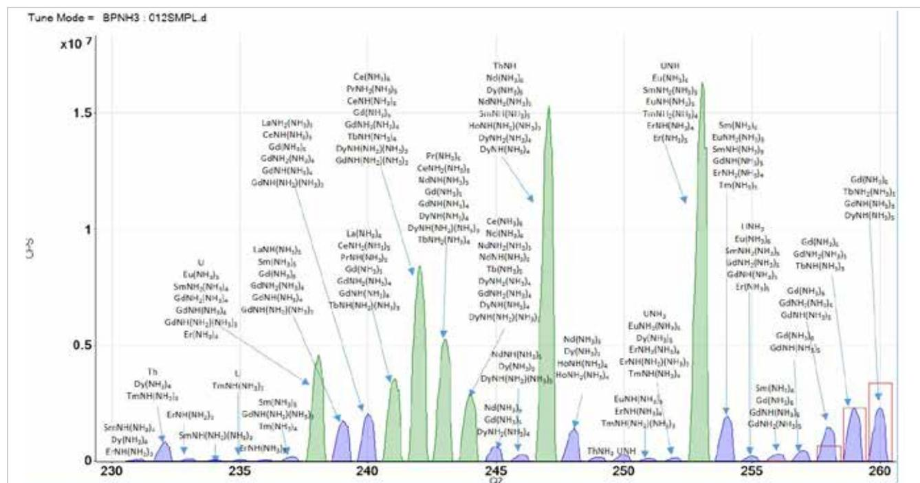
**Figure 5.** Mass spectrum of the mineral sample acquired under Single Quad Bandpass mode using ammonia as the reaction gas. The poor fit of the measured Hf isotopic pattern (far right) illustrates the interferences that occur in Single Quad mode. Some examples of cell-formed ammonia cluster ions are shown.
