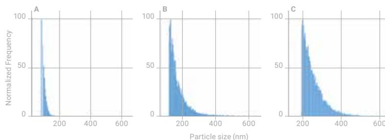
**Figure 3.** Comparison of size distributions for Fe NPs as  $\text{Fe}_2\text{O}_3$  in the three asphaltene samples: A, B, and C. Modified with permission from J. Nelson et al., *Energy Fuels*, 2017, 31 (11), 11971–11976. © 2017 American Chemical Society.
