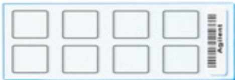
Our 8-plex format offers eight arrays, each with 15,000 probes. These arrays provide a cost-effective tool for the targeted profiling of a large number of samples.
