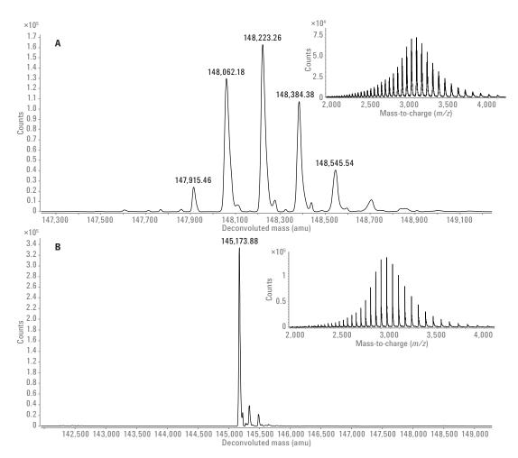
Figure 3. A) Deconvoluted spectrum of intact trastuzumab. B) Deconvoluted spectrum of deglycosylated trastuzumab. The inset shows the raw mass spectra of the analyte.
