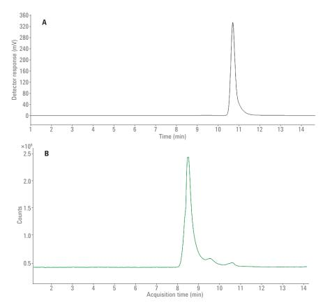
Figure 2. Comparison of SEC analysis of trastuzumab A) with PBS and Agilent 1260 Infinty Bio-Inert Quaternary LC and DAD detection, and B) with ACN/water/FA (50/49/1) and the Agilent 1290 Infinity II LC and MS detection (TIC signal).
