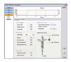
If the CIS is operated with GERSTEL ePneumatics, the MAESTRO Method screen provides an "at-a-glance" graphical display of all parameters including split ratio and resulting flows.
