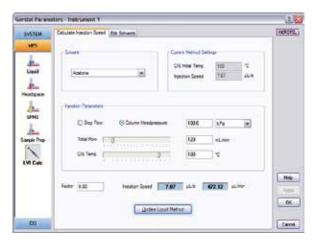
The LVI Calculator is an integral part of the MAESTRO Software. After selecting the solvent from a pull-down menu and entering the injection volume and column flow, a set of optimized method parameters are suggested, which can be transferred to the method by mouse click.
