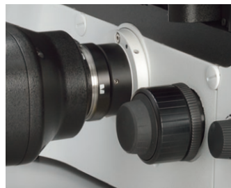
Imaging port with large 25 field number
