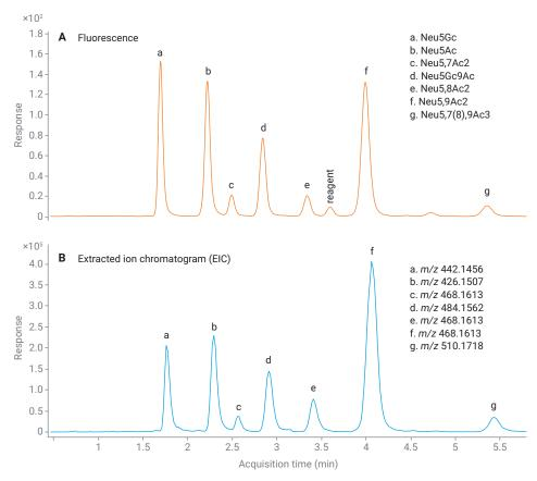
**Figure 2.** UHPLC chromatogram of DMB-labeled SARP. (A) fluorescence; (B) extracted ion chromatogram of DMB-labeled sialic acid species,  $[M+H]^{1+}$ .
