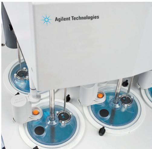
The Dosage Delivery Module (DDM) can be activated manually or automatically for convenient, repeatable dosage form introduction.
