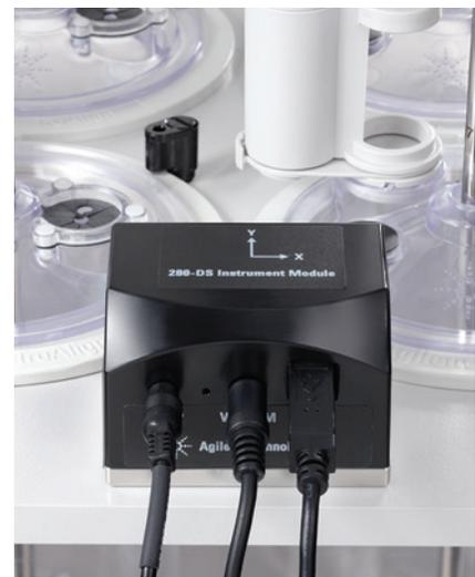
Use the 280-DS Instrument Module and Dissolution Workstation Software to monitor vibration during your dissolution tests. Learn more about qualification with the 280-DS at [www.agilent.com/lifesciences/280-DS](http://www.agilent.com/lifesciences/280-DS).
