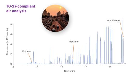
**This analysis of a 5 ppb 65-component VOC standard** demonstrates the ability of Centri to monitor a wide range of 'air toxics' in accordance with US EPA Method TO-17.
