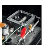
If applicable, the trap is thermally desorbed at up to 100°C/s to inject the sample into the GC-MS as a narrow band.
