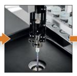
The probe is removed from the vial, and a wash/dry station removes residual sample matrix.
