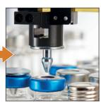
The headspace vials are re-sealed with special caps to avoid contamination of laboratory air.
