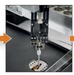
The probe is thermally desorbed and vapours transferred to the focusing trap.
