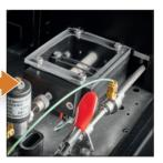
If applicable, the trap is thermally desorbed at up to 100°C/s to inject the sample into the GC-MS as a narrow band.
