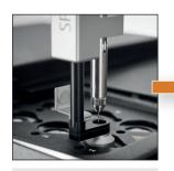
The SPME fiber is normally positioned in the sample headspace and incubated/agitated to facilitate extraction.
