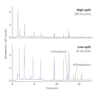
A wide concentration range is achieved for this analysis of off-odours in wine, using immersive sampling with HiSorb probes. Any risk of detector overload is avoided by first using a high split, and the re-collected sample is then run at a lower split to detect two tracelevel 'Brett' compounds.
