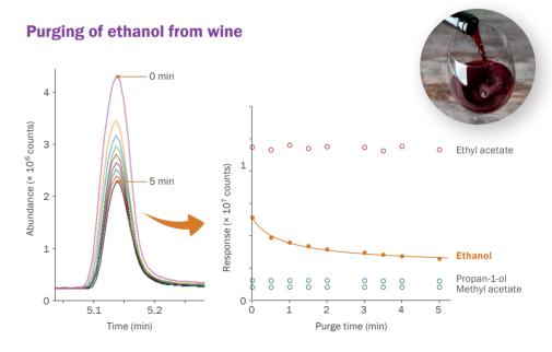
**Selective purging of interferents** is a key benefit of trap-based focusing on Centri, as illustrated here for red wine analysed in headspace–trap mode. Increasing the purge time from 0 to 5 minutes results in a steady decrease in the amount of ethanol reaching the GC-MS, without affecting target compounds eluting nearby.
