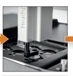
Headspace vapour is withdrawn. Overlap mode optimises productivity for the incubation & sampling of multiple HS vials.
