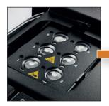
The sample vial is incubated/agitated to speed up analyte equilibration.
