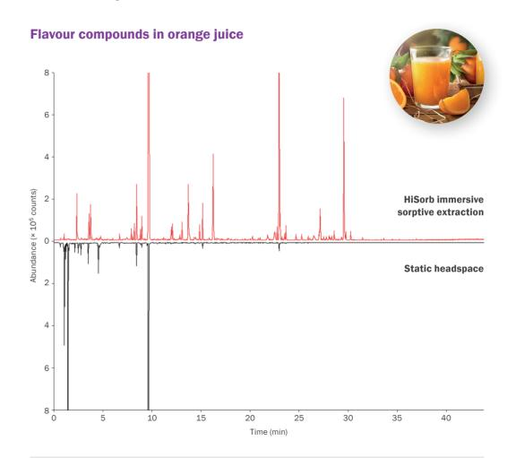
**Improved sample characterisation** is possible over a wide volatility range by harnessing the ability of Centri to analyse samples using various injection techniques. In this example of orange juice, static headspace provides information on the most volatile components contributing to product aroma, while immersive sorptive extraction using HiSorb probes adds detail on less volatile flavour components.
