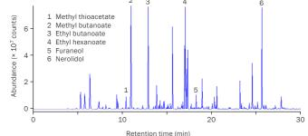
**Aroma-profiling foods and beverages** is widely studied using TD. In this example, Markes' Micro-Chamber/Thermal Extractor is used to quickly profile a range of aroma compounds from strawberries in a single run.
