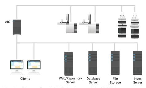
Figure 3 4-Server topology: For high-load environments with multiple AICs
