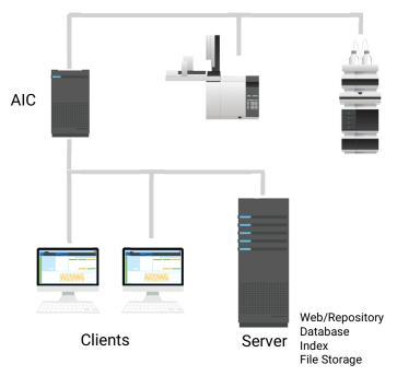
Figure 1 All-in-one topology: Clients and AIC link to one server
