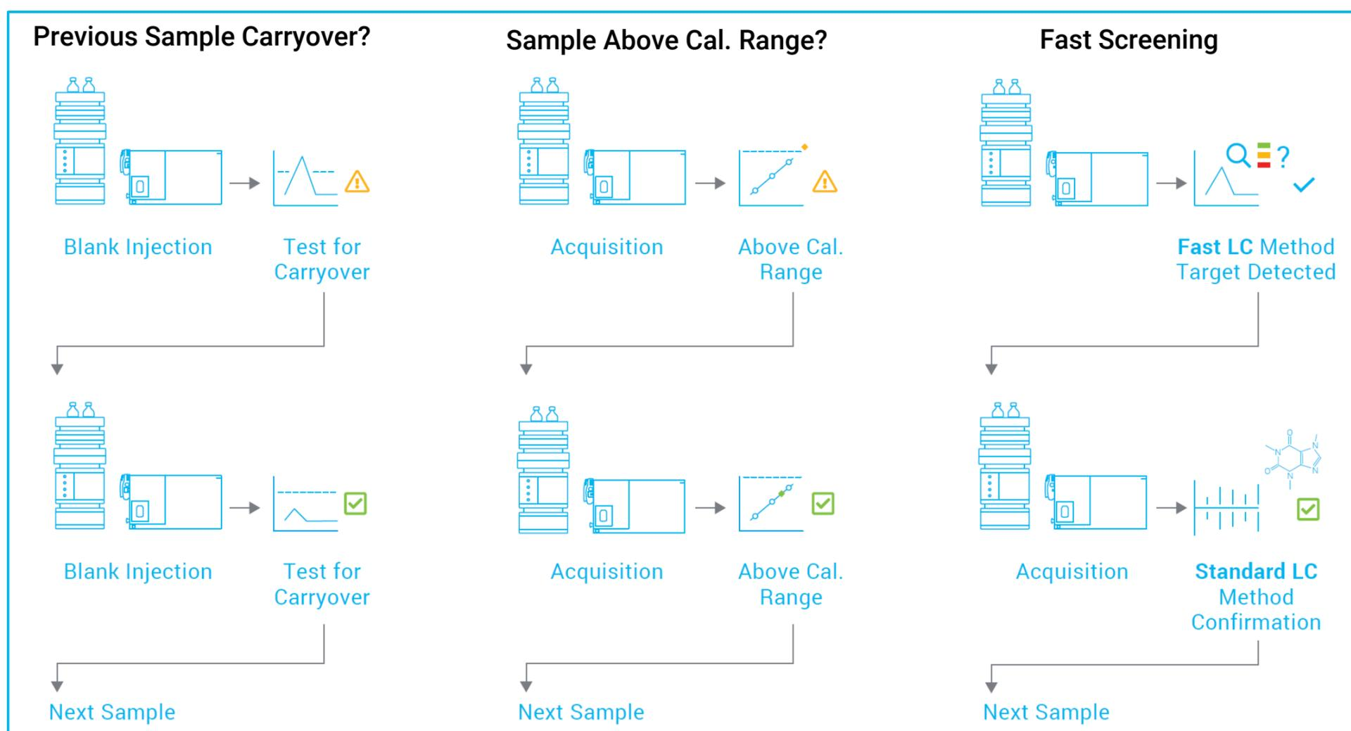
Figure 1: Intelligent Reflex (iReflex) Workflow logic.
