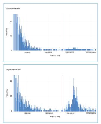
**Figure 3.** Frequency distribution plots for SiO<sub>2</sub> NPs. Top, equal bin size. Bottom, weighted bin size.
