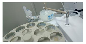
Figure 1. Agilent I-AS autosampler with Organo UPW flowing rinse port system.
