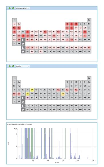
Figure 2. Top and middle: ICP-MS MassHunter IntelliQuant concentration heat map and outlier flags indicating possible spectral overlap. Bottom: Quick Scan full mass spectrum enables identification and confirmation of semiquantitative results for uncalibrated elements.
