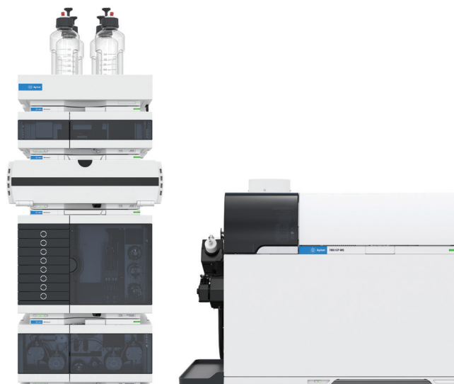
Figure 1. Agilent 7900 ICP-MS coupled to an Agilent 1260 HPLC: one example of the integrated speciation systems available from Agilent.
