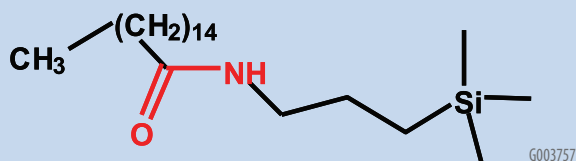
Figure 10. Structure of Ascentis RP-Amide
