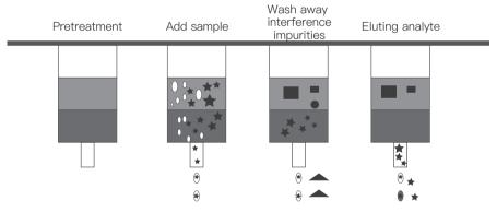
Pre-rinse the activate the columella to ensure the correct method.
