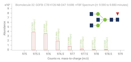
The released glycans results include spectra annotated with the glycan structure and theoretical isotope distribution. The Agilent Find-by-Formula algorithm takes advantage of the glycan tendency to ionize with multiple adducts, resulting in finding species, such as M+H+Na, and giving greater specificity.
