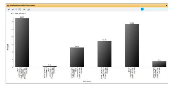
Relative quantitative results of glycoforms are displayed as histogram plots, allowing you to monitor a process.
