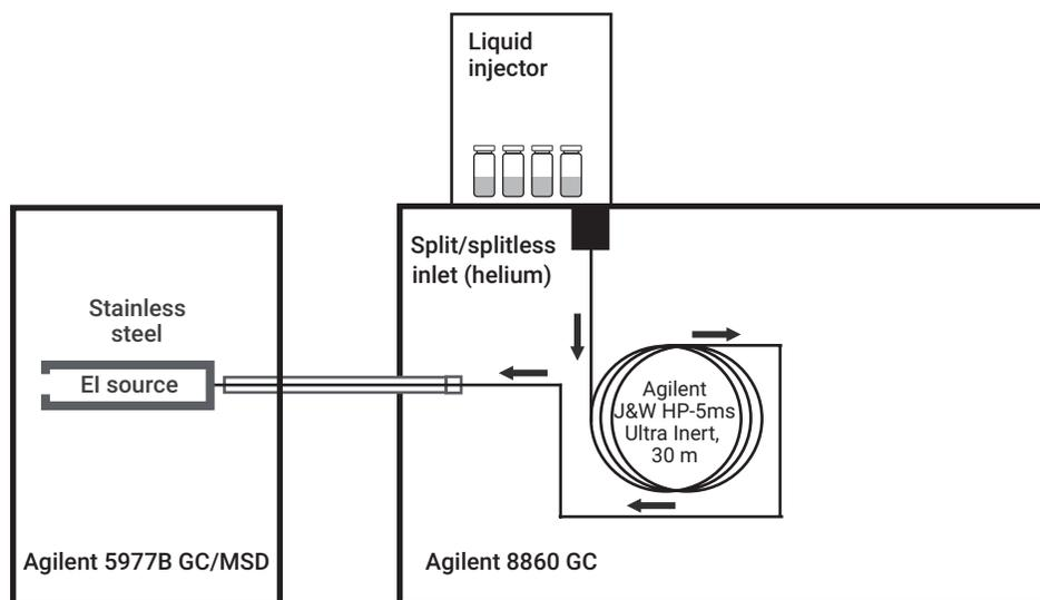
Figure 1. Configuration of the Agilent 8860 GC and Agilent 5977B GC/MSD systems.
