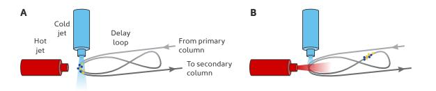
**Stage 2:** The process repeats at the second modulation point, (**A**) focusing the analytes into a narrow band prior to (**B**) injection onto the secondary column for sharp, modulated peaks.
