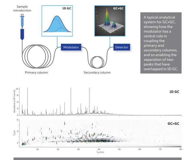
For this complex sample, GC×GC resolves about 10 times as many compounds as 1D GC – typical of the improvement in separating power that a well-chosen modulator can provide.
