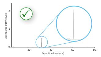
**Uncover hidden details effortlessly.** As shown by this example, Smart Subtract suppresses small relative changes between chromatograms, resulting in a clean background that reliably highlights only the key differences (in this case the single spiking compound).
