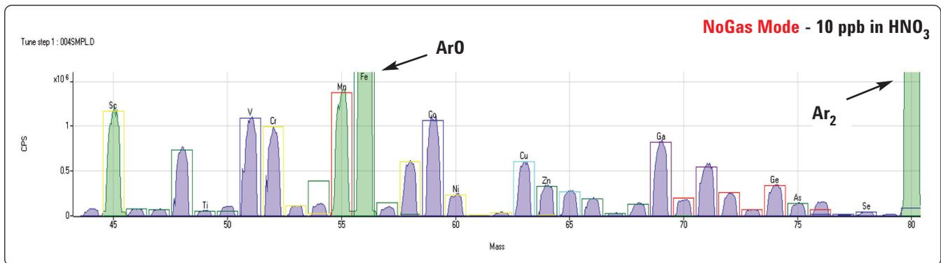
Figure 5a. Relative sensitivity for analytes from Sc to Se in no gas mode.
