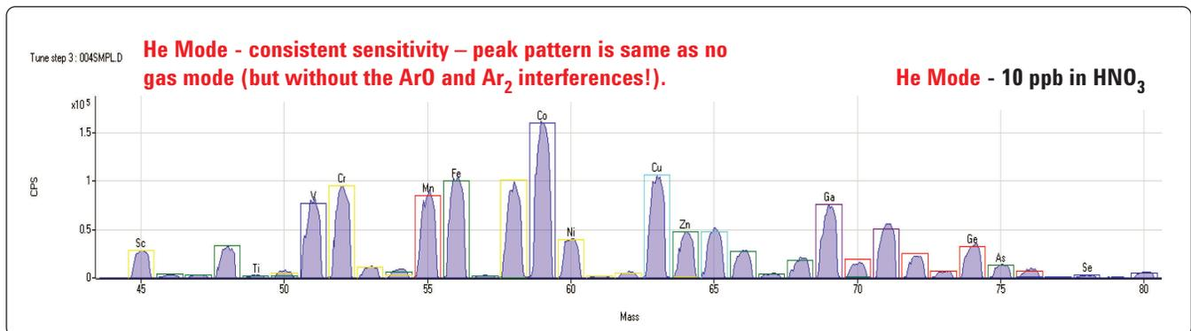
Figure 5b. Relative sensitivity for analytes from Sc to Se in He mode.
