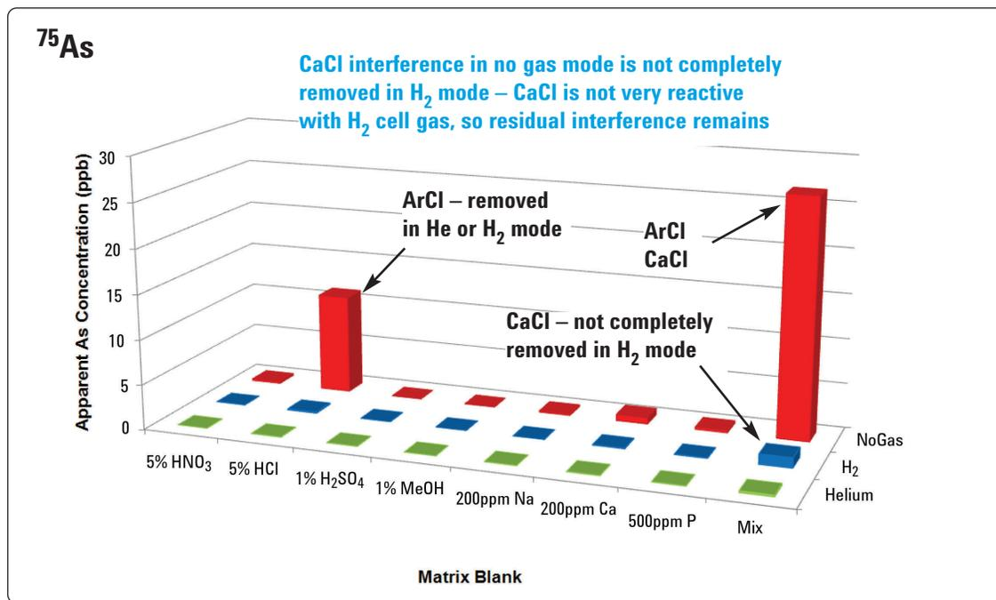
Figure 1. Comparison plot of <sup>75</sup>As BEC vs sample matrix for three cell modes.
