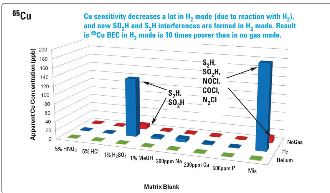
Figure 4. Comparison plot of  $^{65}\text{Cu}$  BEC vs sample matrix for three cell modes.
