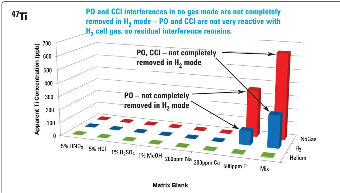
Figure 2. Comparison plot of <sup>47</sup>Ti BEC vs sample matrix for three cell modes.
