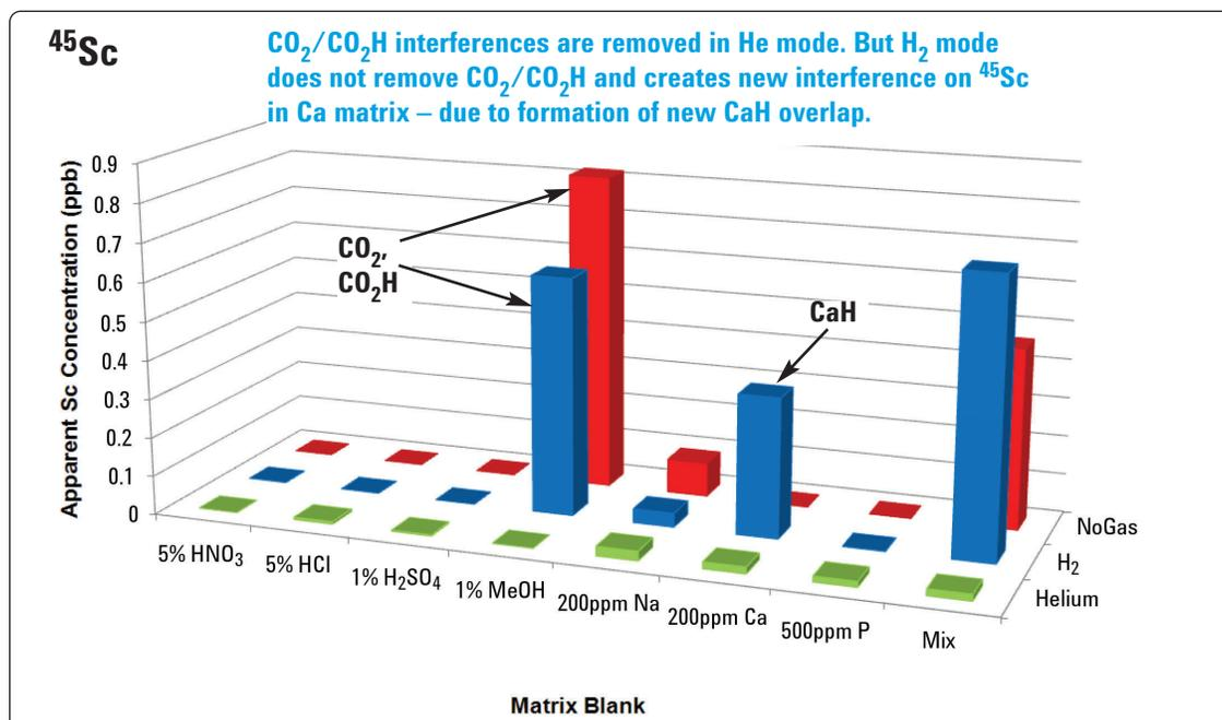
Figure 3. Comparison plot of <sup>45</sup>Sc BEC vs sample matrix for three cell modes.
