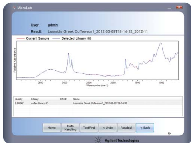
Figure 4. Correct identification of an unknown coffee sample by the Agilent MicroLab FTIR software
