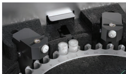
Autosampler carousel with vial sensor and inlet/outlet lifts
