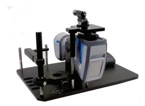
An optional instrument stand is available for using the instrument in a fixed position for development of methods and models. Stages are designed to complement each sampling interface. Pressure devices are also provided for ATR stages dependent on the ATR crystal material.
