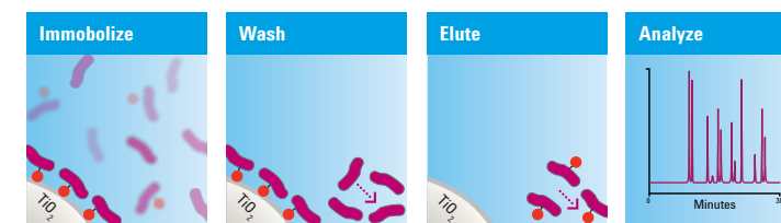
Enrichment and analysis of phosphopeptides with a \text{TiO}_2 workflow.
