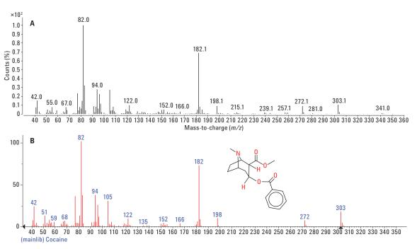
Figure 2. Mass spectrum of 100 pg cocaine spiked in serum (A) compared with NIST spectrum (B). Cocaine is the first hit in NIST. The match factor is 810 (good) [3], and is differentiated from pseudococaine, which has a match factor of 788 (fair). The equivalent concentration is 5 ng/mL based on complete recovery. Excellent NIST library matches ( $\geq 900$ ) for cocaine as a first hit are returned at concentrations above this level.
