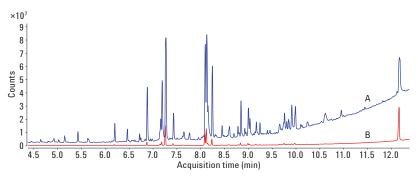
Figure 1. Overlay of TICs of 500 pg standard in serum using A) HES autotune, and B) extractor source etune.
