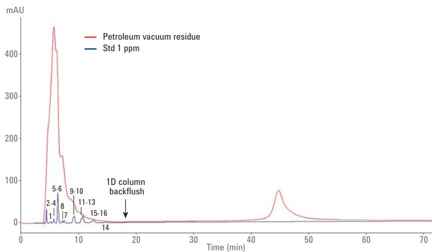
Figure 3. Analysis of the sample and a PAH standard mixture (1 ppm in iso-octane/cyclohexane 1/9 v/v, 2  $\mu$ L injected) with the first dimension normal phase method on the Polaris NH2 column with heptane as the mobile phase. Detection: DAD 254 nm.
