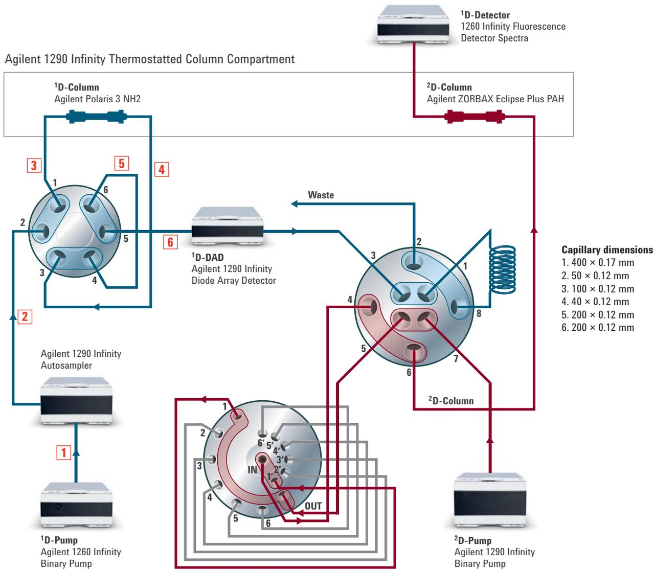
Figure 1. Configuration for multiple-heart cutting 2D-LC. Capillary dimensions:
