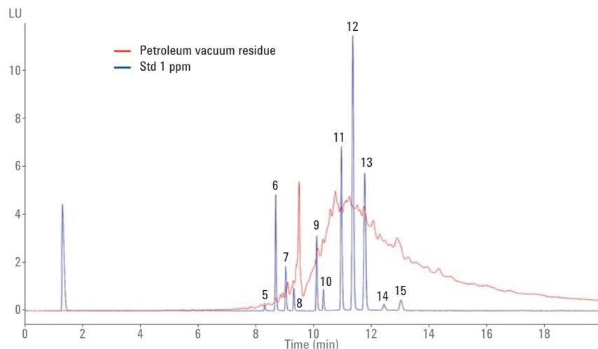
Figure 4. Analysis of the sample and a PAH standard mixture (1 ppm in acetone, 2  $\mu$ L injected) with a typical PAH method using a water/acetonitrile gradient. This method is different from the second-dimension method in the MHC setup. Flow rate: 1.5 mL/min, gradient: 5 to 100 % acetonitrile in 10 minutes, detection: FLD, excitation/emission 260/440 nm.
