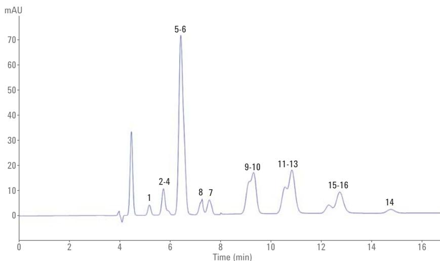
Figure 2. Analysis of a PAH standard mixture (1 ppm in iso-octane/cyclohexane 1/9 v/v, 2 μL injected) with the first dimension normal phase method on the Polaris NH2 column with heptane as mobile phase. Detection: DAD 254 nm.
