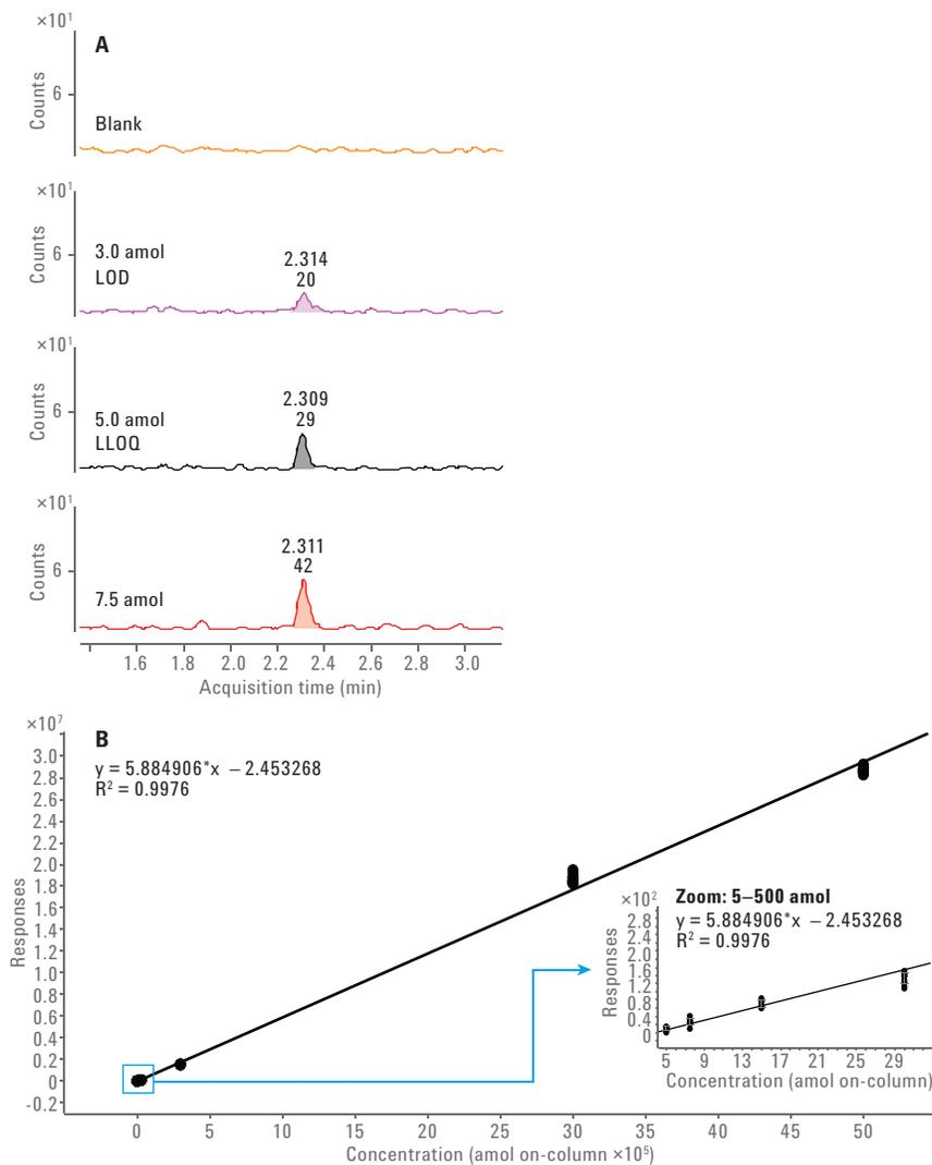
Figure 1. Standard flow LC/MS results for the peptide standard LVNEVTEFAK in 10 fmol/ $\mu$ L trypsinized enolase. A) Stacked extracted ion chromatograms showing the LOD and LLOQ. B) Standard curve with inset showing detail for the range of the curve from 5 to 500 amol.
