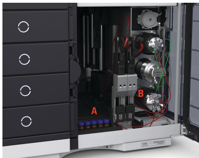
Figure 3. Required changes for PFAS analysis to the Agilent 1260 Infinity II or the Agilent 1290 Infinity II multisampler. A) Vials and caps; B) rotor seal. If the LC has been used for prior PFAS analysis, then replace stator head too. Note: Figure depicts dual needle assembly, but analysis can be performed with just single needle setup.
