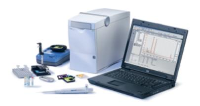
The Agilent 2100 Bioanalyzer system is a versatile system for sizing, quantification and quality control of DNA, RNA, proteins and cells on a single platform.
