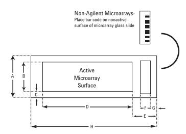
Dimensions for non-Agilent glass slides and array placement for image analysis on Agilent's microarray scanner
