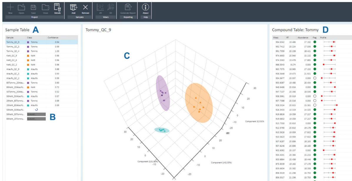
Figure 6. Classifier 1.0 results are displayed in the Sample Table (A) and unanalyzed samples are queued (B). The individual sample details can be viewed by PCA plots (C) or feature details in the Compound Table (D).
