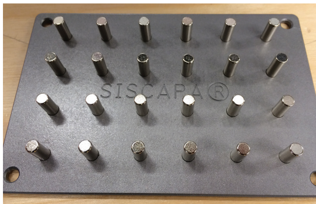
Figure 4. SISCAPA custom magnet array used for washing of magnetic beads.
