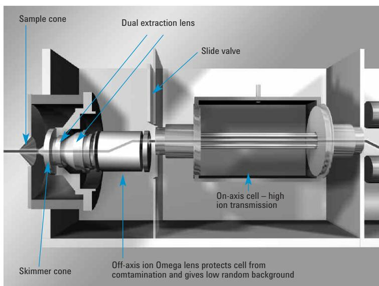
**Figure 12:** Schematic of Agilent Octopole Reaction System
