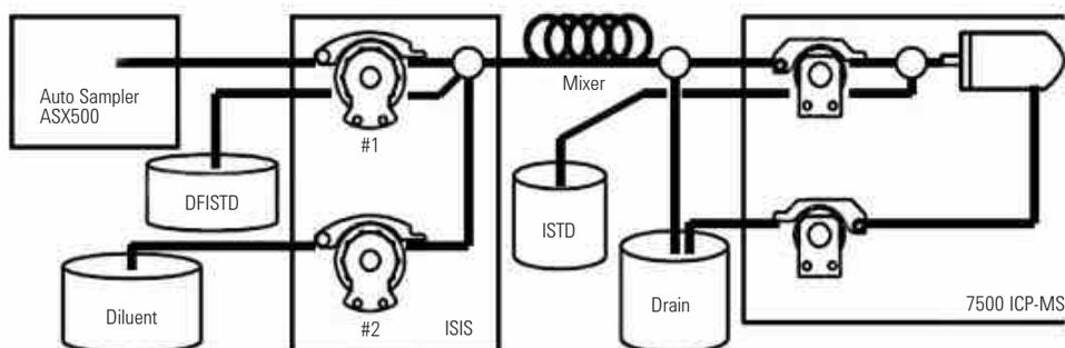
Apart from the time saving by automation, the main advantage of this approach over syringe-pump systems is that extra empty sample vessels are not required and the sample rack of the autosampler can be filled to maximum capacity.
