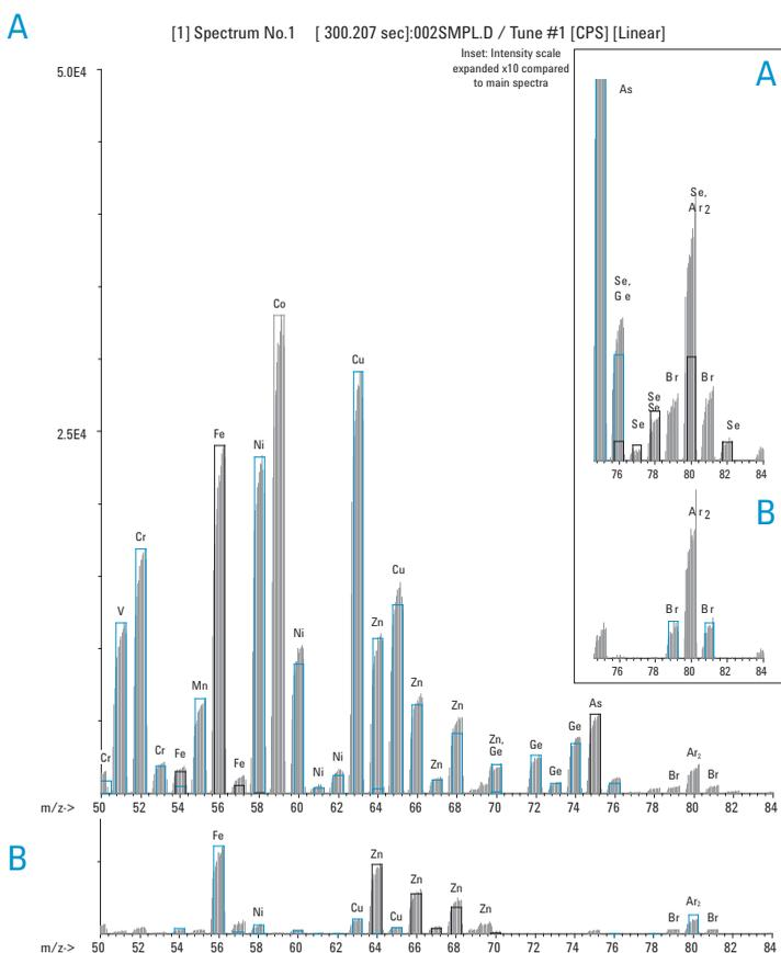
**Figure 7:** High matrix sample in He mode, unspiked (b) and spiked at 5ppb for V, Cr, Fe, Mn, Ni, Co, Cu, Zn, Ge, As and Se (a). Intensity scale of 5.0E4 (5.0E3 for inset spectra)
