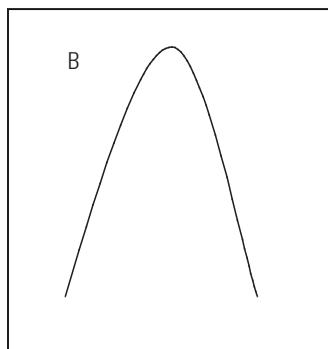
**Figure 2:** The effect of sampling rate (scan rate) on chromatograph peak shape. (a) – too few scans to accurately define the peak shape resulting in imprecise and inaccurate quantification, (b) – sufficient number of scans for accurate quantification
