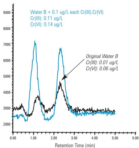
**Figure 8:** Analysis of Cr (III) and Cr (VI) in natural mineral water (unspiked and spiked with 0.1 ug/mL each Cr (III) and Cr (VI)), by ion chromatography-ICP-MS. Mobile phase: 5 mM EDTA (pH 7.0); Flow rate: 1.2 mL/min; Injection volume 500 µL; Sample addition 5 mM EDTA (pH 7). [Agilent application note 5989-2482EN]
