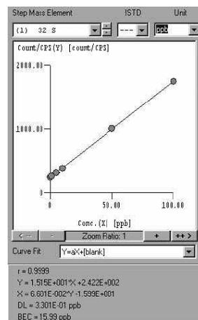
summarizes the analysis of the Chinese Certified Reference Material GBW 08501 Peach Leaf using an Agilent 7500ce ICP-MS.
