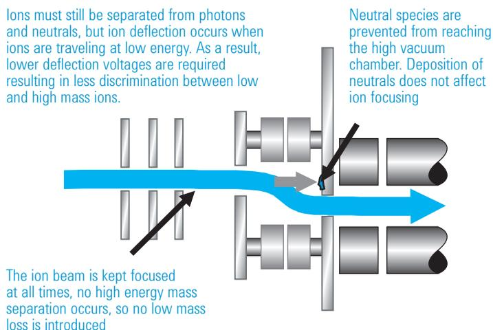
**Figure 11:** Schematic of Agilent off-axis ion lens design
