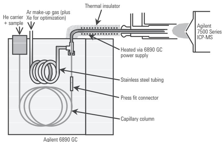
lower RF power settings. Typical RF power when using the Agilent GC interface is 600-900 watts, and these sampling conditions are by no means “cool plasma” providing efficient ionization of poorly-ionized elements such as P, S and the halogens.
