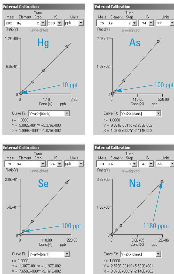
**Figure 1:** Illustration of wide dynamic range and high sensitivity of the 7500ce ORS. Simultaneous measurement at 10 ppt and >1000 ppm. Calibration ranges: Hg: 10 ppt - 2 ppb, As: 100 ppt - 200 ppb, Se: 100 ppt - 200 ppb, Na: 50 ppb - 1180 ppm.
