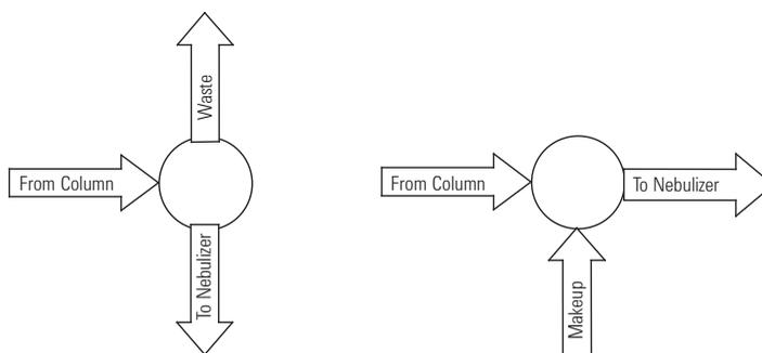
**Figure 4:** Open split (left) and makeup flow (right) configurations for matching nebulizer flow to column flow in LC-ICP-MS
