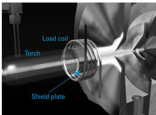
**Figure 3:** ShieldTorch System - Agilent 7500 Series
