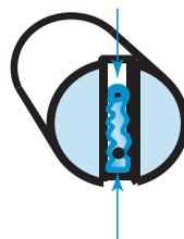
**Figure 4:** Schematic of Agilent High-Solids Babington nebulizer
