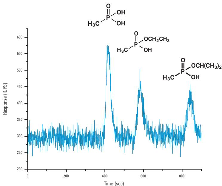
**Figure 5:** Reverse phase ion pairing HPLC-ICP-MS analysis of chemical warfare agent metabolites; EMPA, IMPA and MPA using phosphorus detection.
