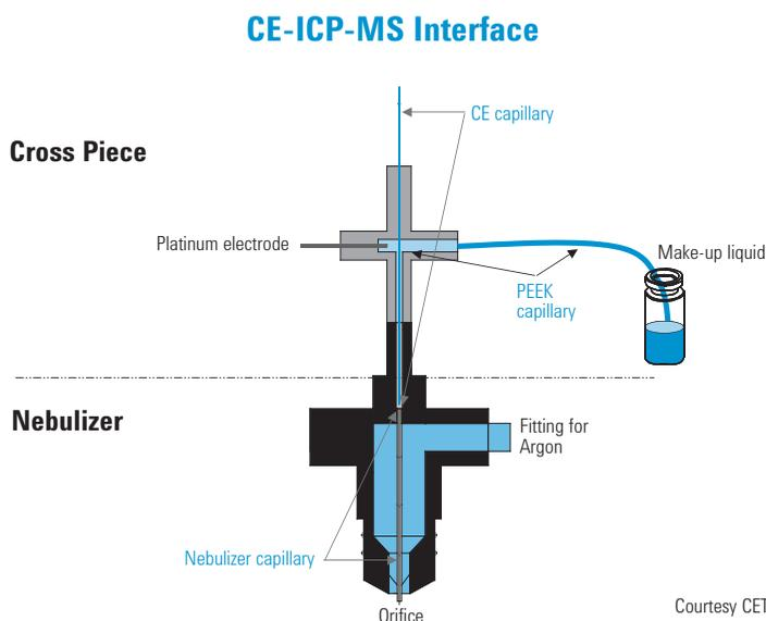
**Figure 9a:** Schematic diagram of Cetac CEI-100 CE-ICP-MS interface
