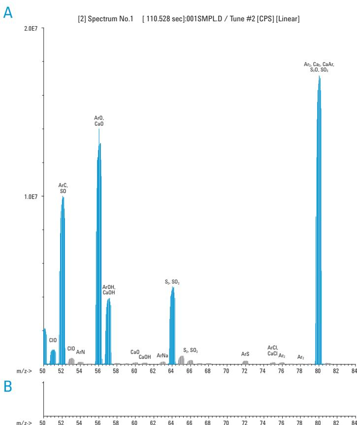
**Figure 5:** High intensity interfering polyatomic ions from high matrix sample (see text for composition) in no cell gas (a) and He cell gas (b) modes, on same intensity scale (2.0E7)
