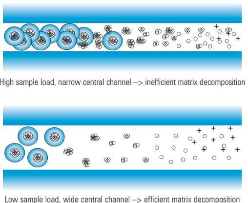
**Figure 9:** Effect of injector diameter on matrix decomposition
