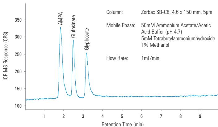
**Figure 6:** LC-ICP-MS analysis of the phosphorus containing herbicides glyphosate, glufosinate and the metabolite AMPA.
