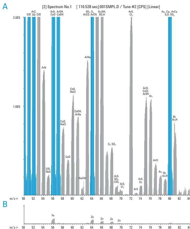
The comparison of the spectra obtained in He mode for the blank (unspiked) matrix and the spiked matrix (all analytes at 5 ng/mL) is shown in Figures 7a and 7b. Note that these spectra are shown on an intensity scale that is a further 40x lower than that used for Figures 6a and 6b, allowing the presence of the contaminant elements (Fe, Ni, Cu, Zn) to be confirmed from their isotopic templates.
