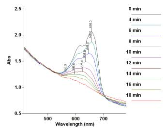
**Figure 2.** Scanning kinetics using fiber optics *in situ* of methylene blue under the exposure of a high-intensity UV lamp (Oriell 500 W Hg(Xe) lamp) over a period of 20 minutes within the range 400 to 800 nm. Labels refect maximum absorbance wavelengths
