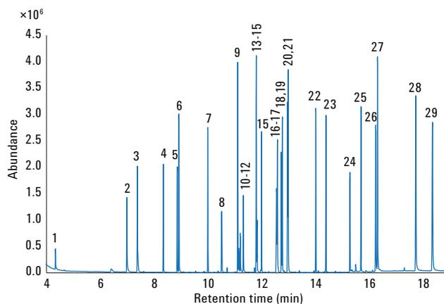
Figure 2. Total ion current chromatogram of 29 components in a semivolatile checkout mixture at 10 ng/component on-column when the Agilent J&W Ultimate Plus deactivated fused silica tubing was used as the GC restrictor for the MS interface (see Table 1 for peak IDs).
