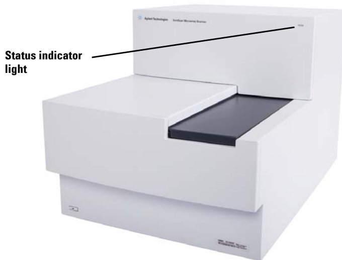
Figure 13 Location of the status indicator light
