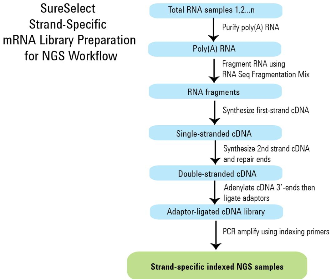
Figure 2 Overall sequencing sample preparation workflow
