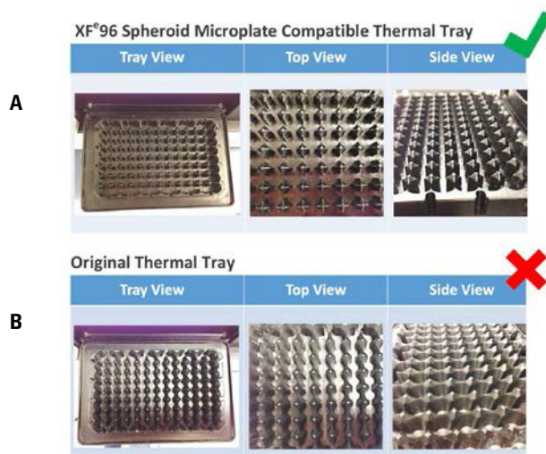
Figure 3 Agilent Seahorse XFe96 Spheroid Microplate-compatible Thermal Tray and Correct Plate Type File
